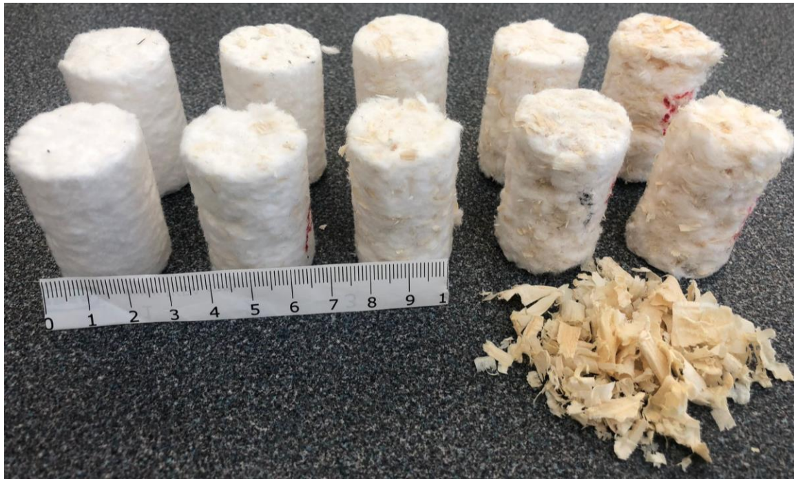
Fig. 1. Samples with increasing CSs content from left to right (S1 to S5). The samples with a lower CP content (sample A) are in the front row. A loose sample of CSs was placed in front of the samples. The samples were cut to size for impedance tube measurements
