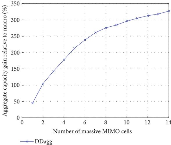
FIGURE 8: Aggregate capacity gain relative to macro-only network.
