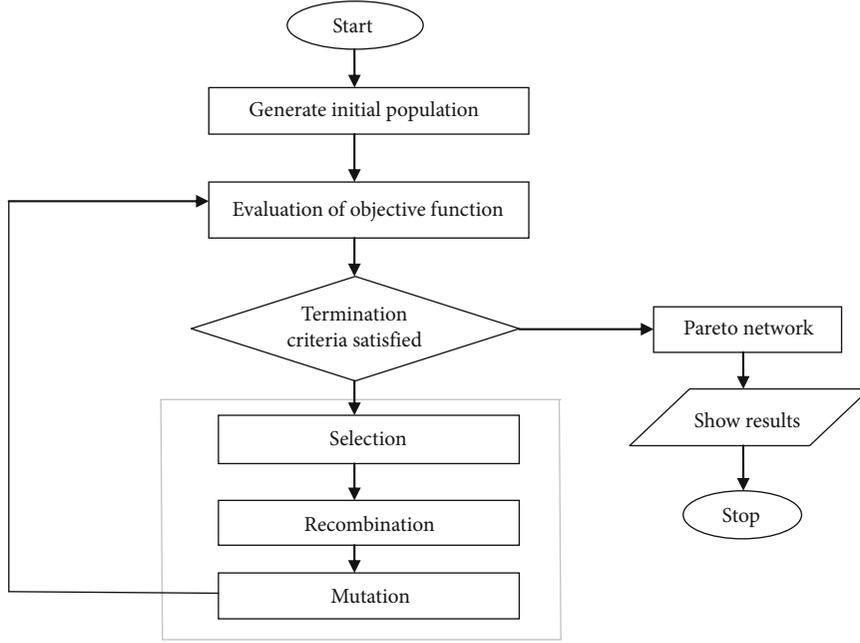
FIGURE 2: Flow chart of genetic algorithm.
