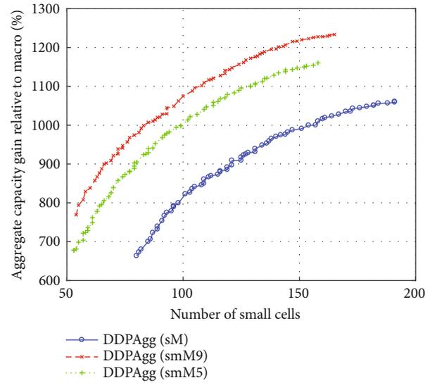
FIGURE 15: Aggregate capacity gain with two-stage optimization.
