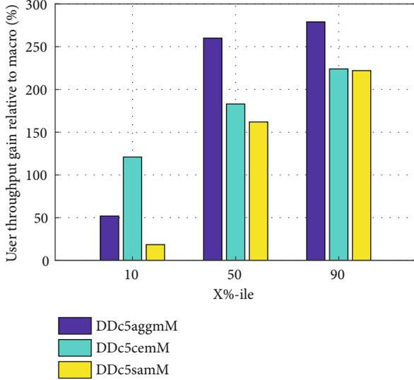
FIGURE 7: 10%-ile, 50%-ile, and 90%-ile user throughput gain.
