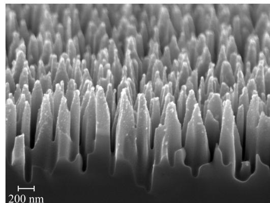
Figure 2: An SEM image of freshly etched b-Si surface.
