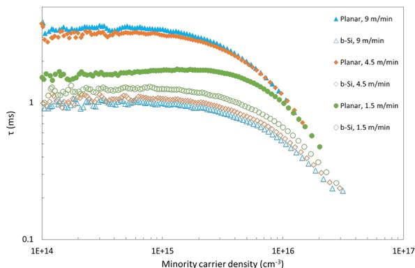
Figure 3:  $\tau$  of planar and b-Si samples coated with SALD with different line speeds.
