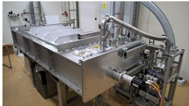
Figure 1: Beneq SCS 1000 SALD reactor installed at the Beneq facilities in Espoo, Finland.
