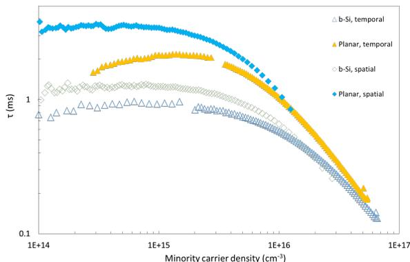
Figure 4:  $\tau$  of planar and b-Si samples coated with SALD and temporal ALD.
