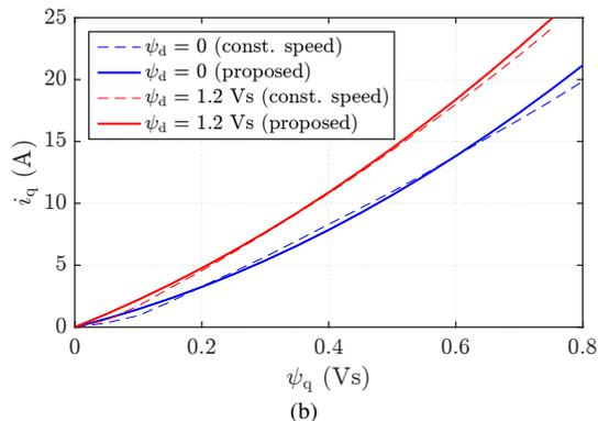
Fig. 6. Currents as functions of the fluxes: (a)  $i_d$  as a function of  $\psi_d$  for  $\psi_q = 0$  and  $\psi_q = 0.6$  Vs; (b)  $i_q$  as a function of  $\psi_q$  for  $\psi_d = 0$  and  $\psi_d = 1.2$  Vs. The dashed lines show the reference data, which has been measured using constant-speed identification. The solid lines show the results from the proposed standstill method.
