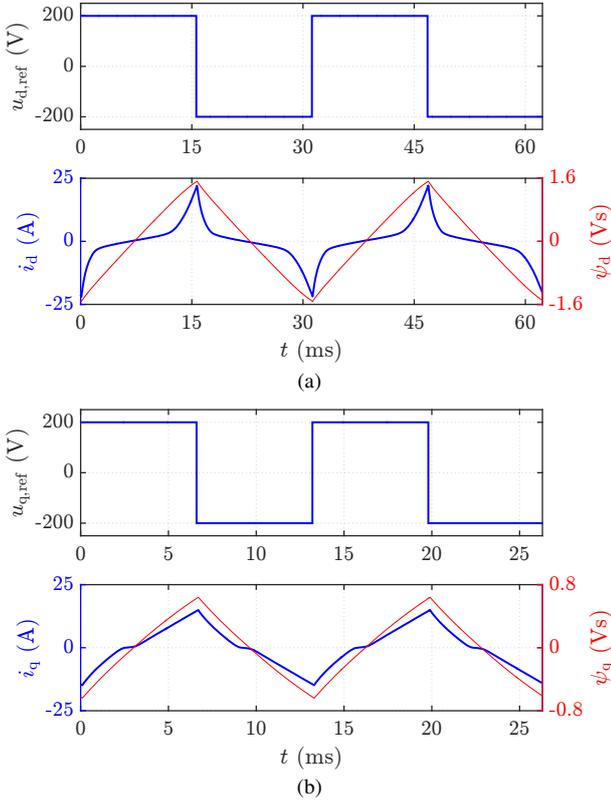
Fig. 2. Measured self-axis test waveforms: (a) d-axis; (b) q-axis. The upper subplots show the voltages. The lower subplots show the measured currents and the calculated fluxes. The parameters are  $u_{d,out} = u_{q,out} = 200$  V,  $i_{d,max} = 20$  A, and  $i_{q,max} = 14$  A. The number of samples is  $N_d = 624$  in the d-axis test and  $N_q = 264$  in the q-axis test.
