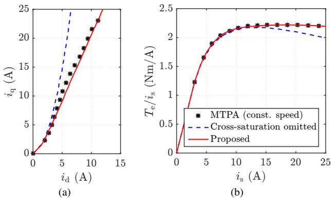
Fig. 7. Comparison of MTPA characteristics: (a) control trajectories; (b) torque factors. The legends given in (b) hold for (a) as well. The current magnitude is denoted by  $i_s$ . The stars show the reference data from the constant-speed method. The red solid curves are calculated using the model (5) and the fitted parameters. In the case of the blue dashed curves, the cross-saturation is omitted by setting  $a_{dq} = 0$ .
