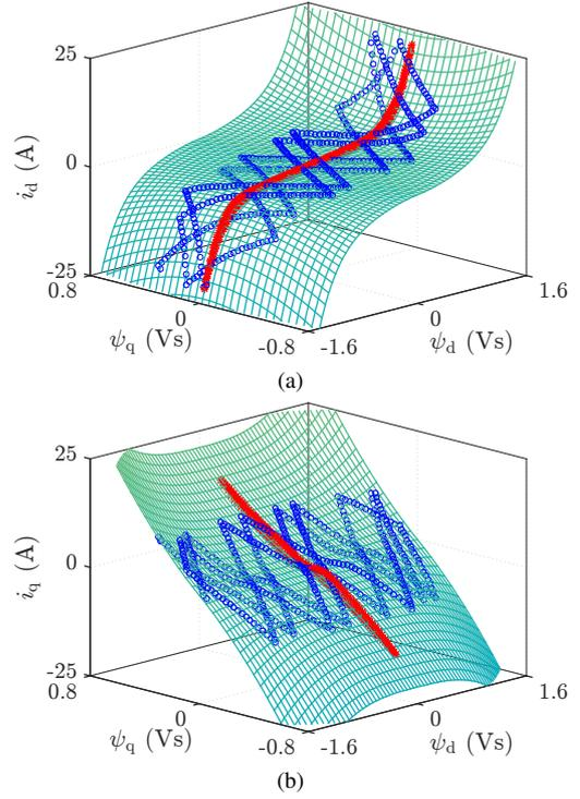
Fig. 5. Currents as functions of fluxes: (a)  $i_d$ ; (b)  $i_q$ . The mesh surfaces correspond to the fitted model (5). The red stars show the measured samples from the self-axis saturation tests, cf. Fig. 2. The blue circles show the measured samples from the cross-saturation test, cf. Fig. 3.
