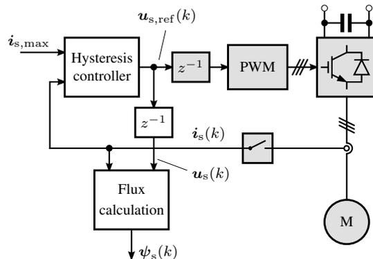
Fig. 1. Sensorless identification setup. The white blocks represent the control algorithm. The grey blocks model the plant: motor, converter, PWM, sampling, and computational time delay  $z^{-1}$ . The vector representation is used:  $\mathbf{i}_s = [i_d, i_q]^T$ ,  $\mathbf{u}_s = [u_d, u_q]^T$  and similarly for other vectors.
