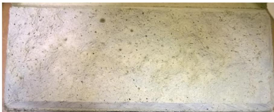
Figure 10. Example of top surface quality of sample 1x14T with dimensions of 170 mm x 60 mm.
