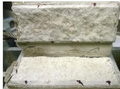
Figure 13. Pilot #3 sample top and bottom samples after loading
