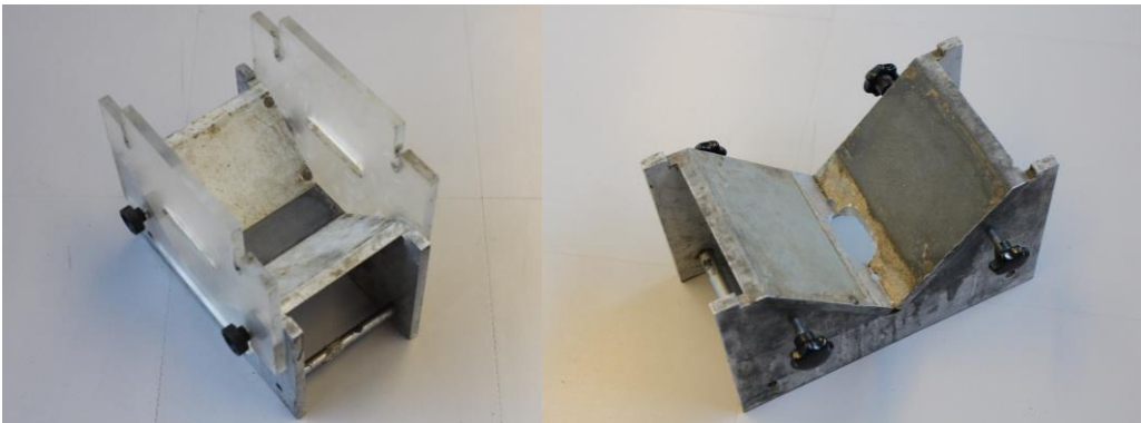
Figure 9a. The aluminum mold with the plexiglass plates. Figure 9b. The casting hole drilled in bottom.
