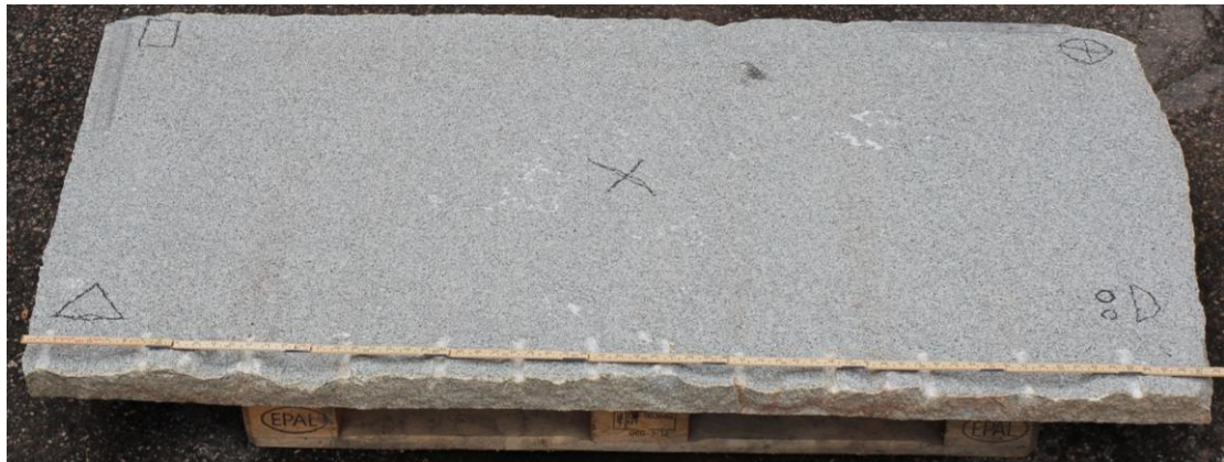
Figure 1. The granitic rock surface with dimensions of 175 cm x 95 cm resting on a pallet
