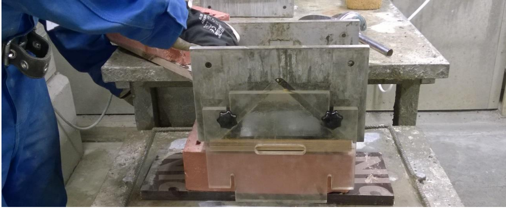
Figure 8. The entire casting mold assembly on top of a vibration table
