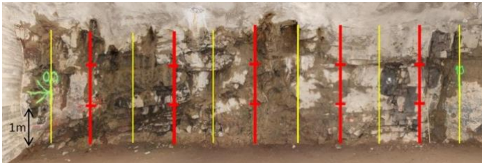
Figure 1. Chainage 00-10 meters with windows (yellow) and skylines (red).
