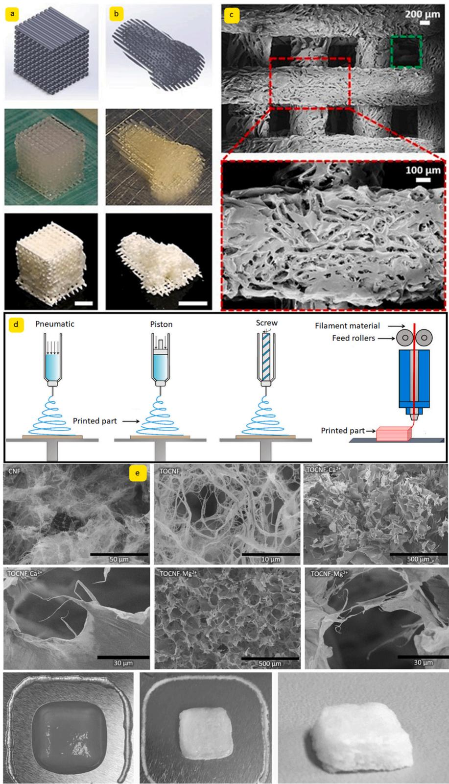
**Fig. 9.** 3D printed dual pore scaffold aerogel with 20 wt% CNC for (a) a cube and (b) a human nose model, and (c) its corresponding SEM images (Li et al., 2017). (d) Different techniques for 3D printing of lignocellulosic-based materials. (e) Representative SEM images of CNF and cross-link CNFs with various metallic cations as inks and their printed samples (Mietner et al., 2021).
