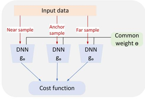
Fig. 2. Triplet network architecture. The three DNN blocks are identical and use common weights [9], [19].
