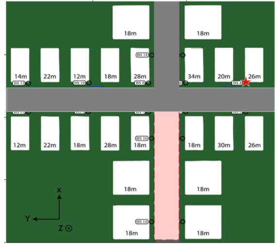
Fig. 3. Simulation layout. The selected street segment is in pink colour. The BS location is indicated by a red star.
