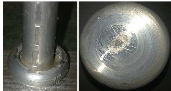
Fig 2: Aluminium tool plunged on to the surface of Mild Steel.
