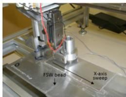
Conductivity measurements were made along a sweep in the X-axis perpendicular to the processed bead, at half thickness.
