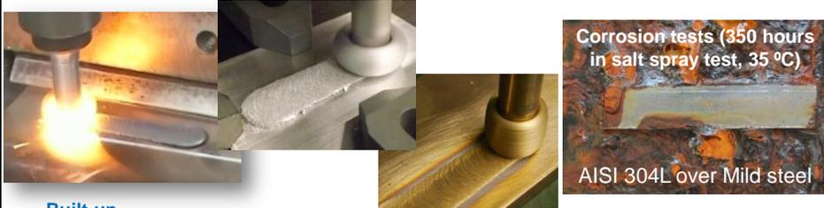
Corrosion tests (350 hours in salt spray test, 35 °C)
