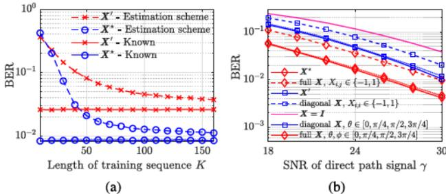
Fig. 4. In (a), BER performance as a function of  $K$  for estimating the optimum full and diagonal signaling matrices. In (b), BER comparison between the optimum  $X$  and discretized signaling matrices.
