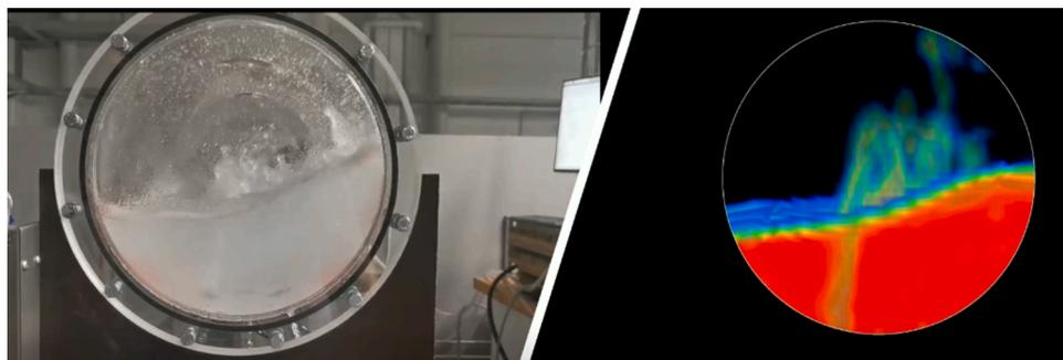
Fig. 3. A screenshot from the numerical model verification video. The water model is shown on the left and the simulated water model on the right. Conditions: air volumetric speed: 140 L/min, operational nozzle number: 5.
