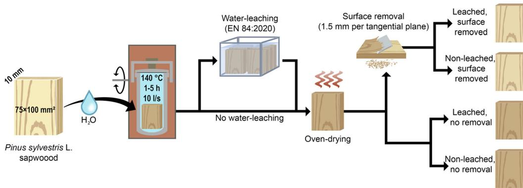
**Figure 1:** Treatment procedure for wood specimens. The prepared specimens were HWE treated in a rotating air-bath reactor at 140 °C for 1–5 h at a liquid-to-solid ratio (l/s) of 10. Afterwards, selected specimens were subjected to leaching and/or surface removal.
