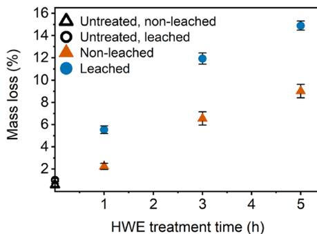
**Figure 2:** Mass loss (%) of wood as a function of HWE treatment time. The error bars indicate the standard deviation.
