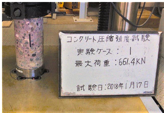
Fig. 20. A photo of the compression experiment of concrete sample.
