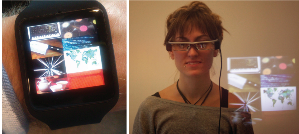
Figure 4: The Digital Self as it appeared on the smartwatch (left) and how it appeared to a user through the HMD (right).
