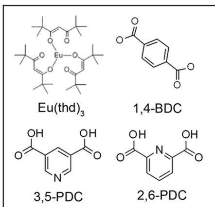
Figure 1. Precursors employed in the present study: tris(2,2,6,6-tetramethyl-3,5-heptanedionato)europium(III) ( $\text{Eu}(\text{thd})_3$ ), 1,4-dicarboxylic acid (1,4-BDC), 3,5-pyridinedicarboxylic acid (3,5-PDC) and 2,6-pyridinedicarboxylic acid (2,6-PDC).
