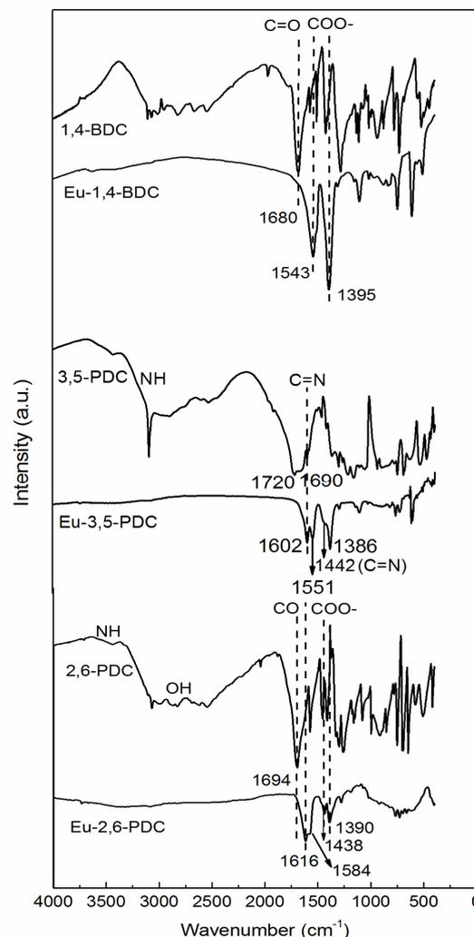
Figure 3. FTIR spectra for the hybrid thin films, Eu–1,4-BDC, Eu–3,5-PDC and Eu–2,6-PDC, and the corresponding organic precursors.
