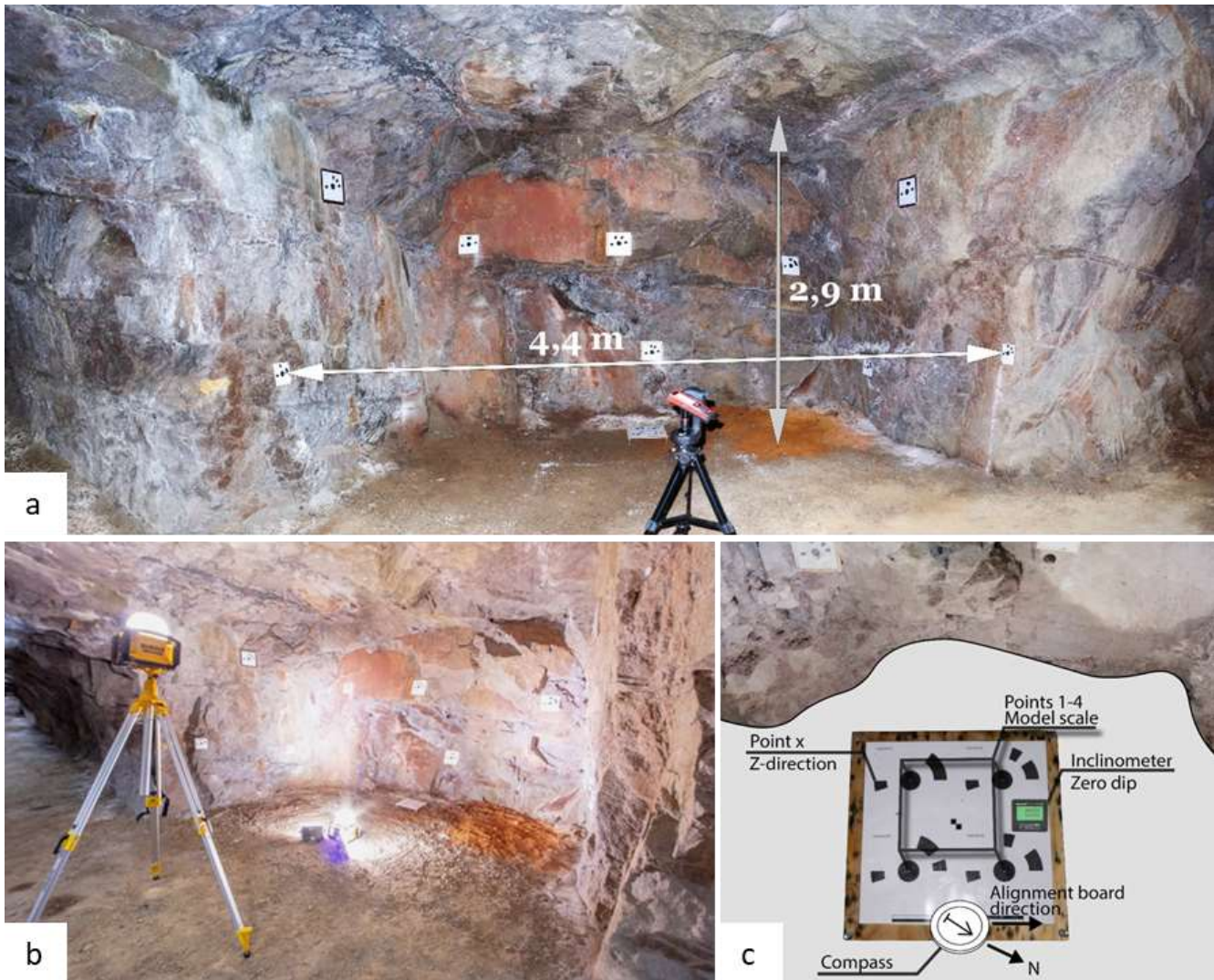
Figure 2. Tunnel drift dimensions (a), the portable lighting setup (b), and the alignment board with control points and known control distances used to scale and orientate the 3D model (c) (modified after Prittinen, 2021).
