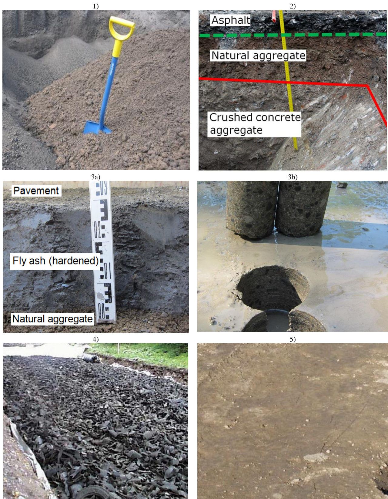
Figure 4 Figures of UUMA-material types 1-5: 1) Bottom ash ( www.uuma2.fi ); 2) Crushed concrete, re-hardened (Dettenborn et al. 2016); 3a) Cement stabilised fly ash; 3b) Fly ash stabilised crushed aggregate (Tarkkio 2014); 4) Shredded tires as a light weight material of street embankment (Forsman et al. 2002); 5) Stabilised surplus clay as a liner (Forsman & Leivo 2007). The explanations for the material types 1-5 are presented in Table 1.
