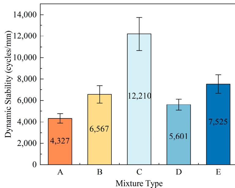
**Figure 10.** Dynamic stability of different asphalt mixtures.
