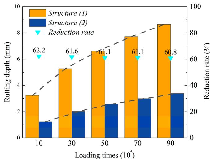
**Figure 14.** Rutting depth for two structures with different loading times.
