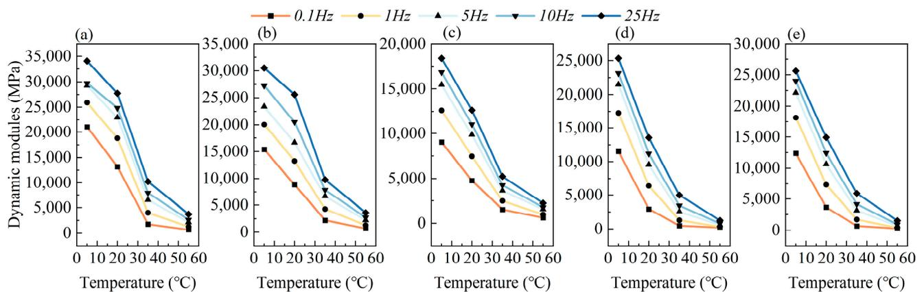
**Figure 6.** Variation of dynamic modulus with temperatures for the five asphalt mixture types at loading frequency ranging from 0.1 Hz to 25 Hz. (a) Mixture A; (b) Mixture B; (c) Mixture C; (d) Mixture D; (e) Mixture E.
