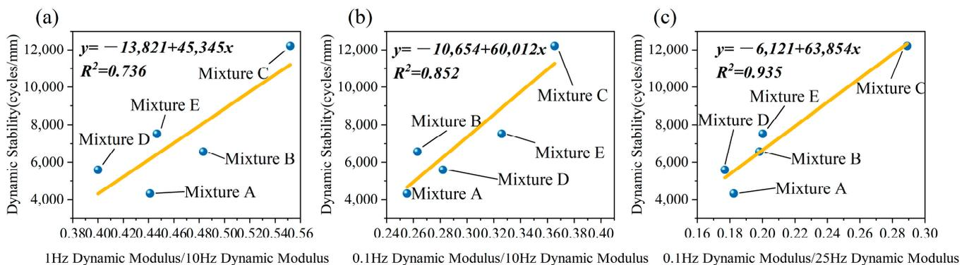
**Figure 12.** Correlation between dynamic modulus at high frequency/dynamic modulus at low frequency and dynamic stability. (a) 1 Hz dynamic modulus/10 Hz dynamic modulus; (b) 0.1 Hz dynamic modulus/10 Hz dynamic modulus; (c) 0.1 Hz dynamic modulus/25 Hz dynamic modulus.
