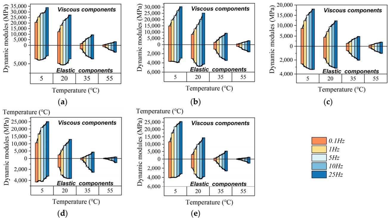
Figure 7. Viscous and elastic components of different mixtures. (a) Mixture A; (b) Mixture B; (c) Mixture C; (d) Mixture D; (e) Mixture E.
