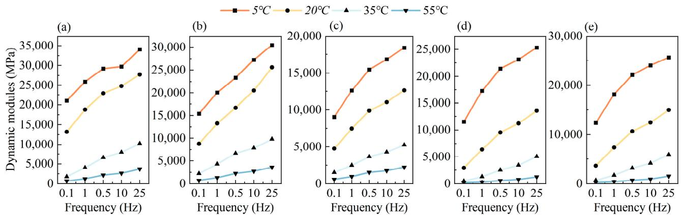
**Figure 5.** Variation of dynamic modulus with loading frequency for the five asphalt mixture types at temperatures ranging from 5 °C to 55 °C. (a) Mixture A; (b) Mixture B; (c) Mixture C; (d) Mixture D; (e) Mixture E.
