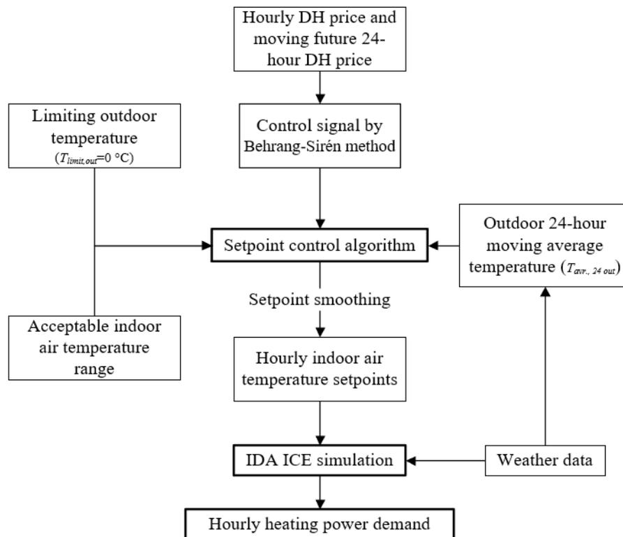
**Figure 2.** Building-level simulation process for DR control.
