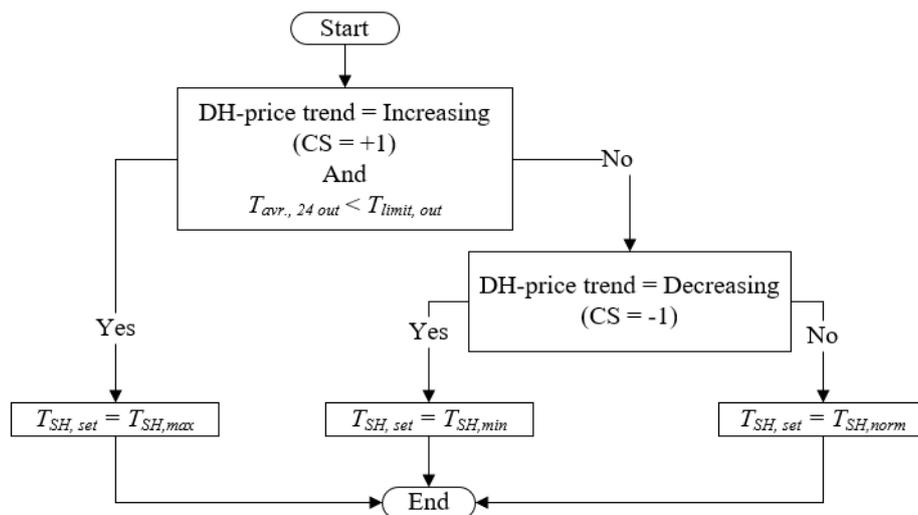
**Figure 4.** Control algorithm for space heating.
