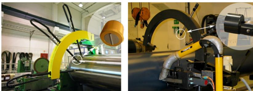
Fig. 7. Four-point measurement devices.
