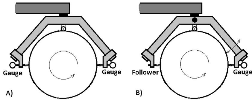
Fig. 3. Modified saddle-type roll callipers for two-point measurement. A) With fixed arms. B) With swing arms.
