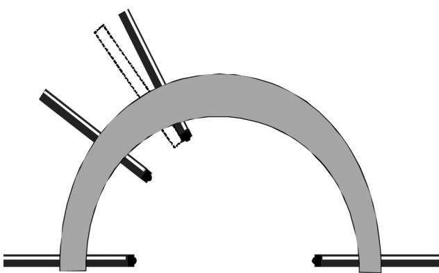
Fig. 12. Alignment/position error of a rod.
