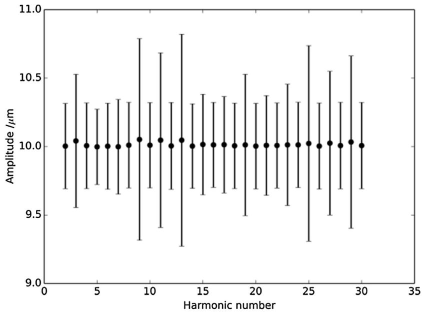
Fig. 15. Output from Monte Carlo simulation, showing standard uncertainties as error bars. This simulation was run with a thermal error ( $\sigma = 1^\circ\text{C}$ ).
