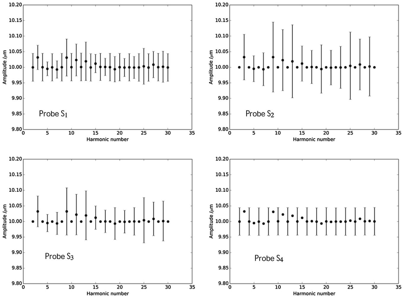
Fig. 16. Outputs from four Monte Carlo simulations for probe error, with the standard uncertainties shown as error bars. These simulations were run with one probe error at a time ( $\sigma = 1\ \mu\text{m}$ ).
