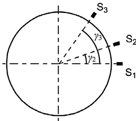
Fig. 4. Orientation and location of the three run-out measurement probes of the Ozono method.
