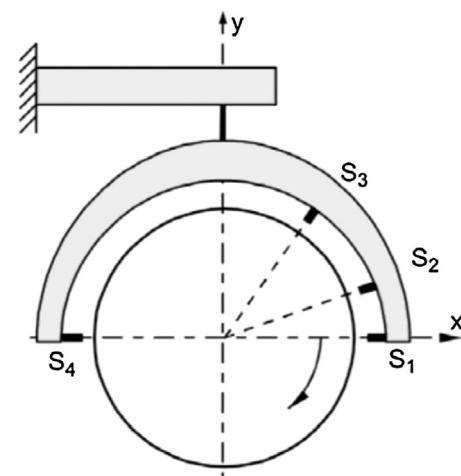
**Fig. 5.** Orientation of probes ( $s_1-s_4$ ) in a four-point measurement system.
