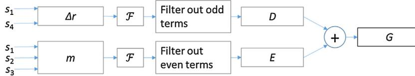
Fig. 6. Principle for the calculation of harmonics of the hybrid four-point method.
