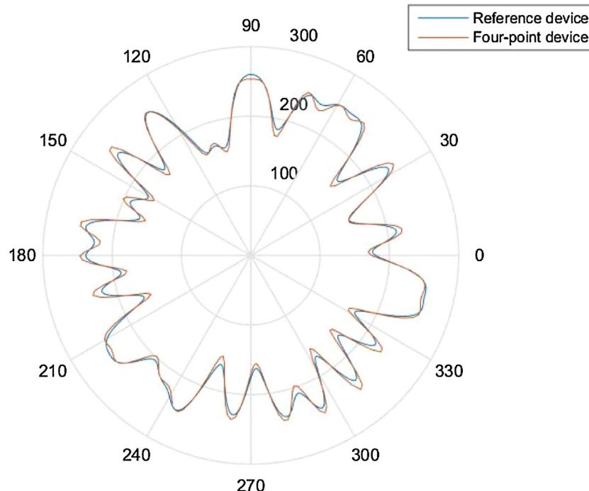
**Fig. 10.** Comparison of four-point measurement device (FFT based harmonic filter UPR 2–30) and reference roundness measurement device (Gaussian 1–30 UPR).
