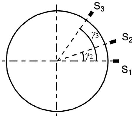
**Fig. 4.** Orientation and location of the three run-out measurement probes of the Ozono method.
