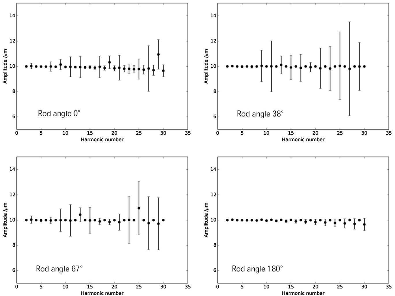
**Fig. 17.** Outputs from four Monte Carlo simulations for alignment error, with standard uncertainties shown as error bars. These simulations were run with one rod alignment error at a time ( $\sigma = 1^\circ$ ).
