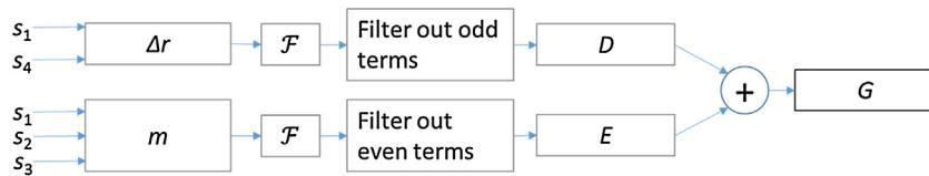
**Fig. 6.** Principle for the calculation of harmonics of the hybrid four-point method.
