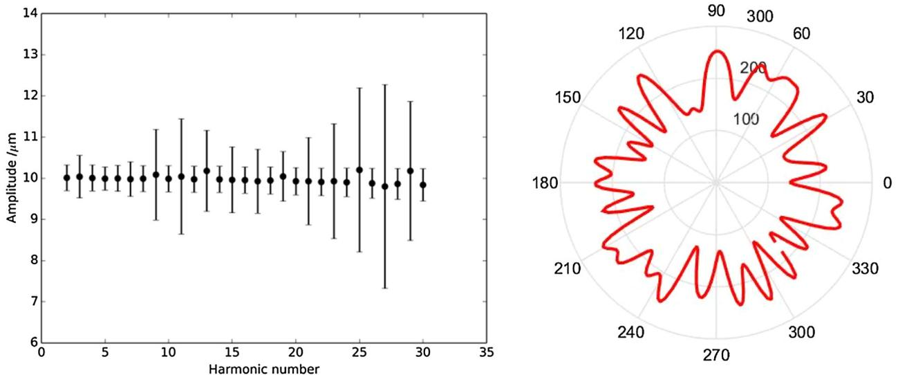
Fig. 14. Output from Monte Carlo simulation where the standard uncertainties are shown as error bars for the harmonics (left) and the average of simulated results as a polar plot (right). This simulation was run with all the error sources specified in Table 1.
