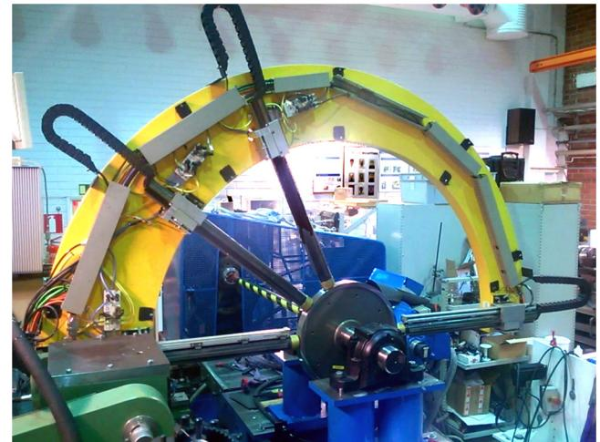
**Fig. 8.** Measurement of a calibration disc with a four-point measurement device. When calibrating a four-point device, the disc is typically attached to a shaft on roller bearings and the shaft is rotated.
