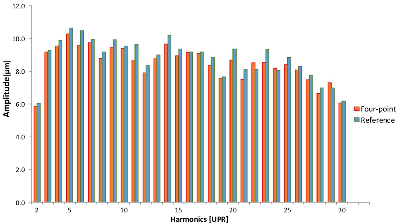
Fig. 11. Comparison of the calculated harmonics of the four-point result and reference roundness result.
