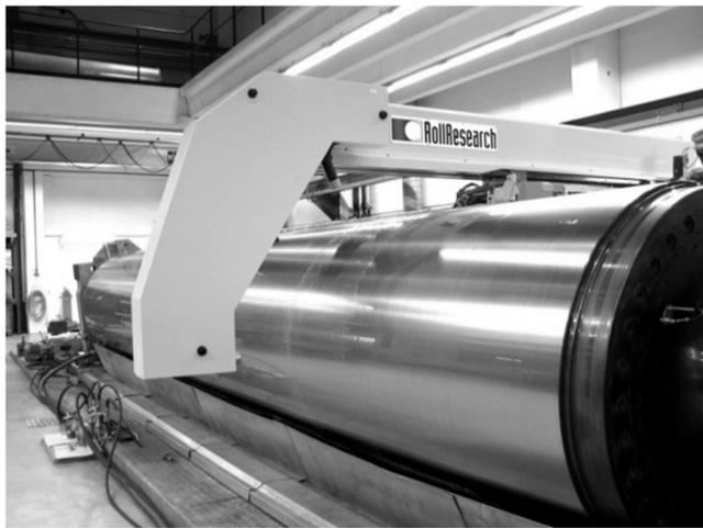
Fig. 1. Four-point roll measuring device of a grinding machine.
