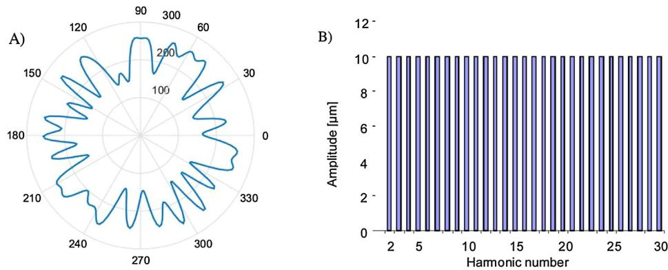
**Fig. 9.** A) Calibration disc profile with harmonics 2–30 UPR (radial scale in  $\mu\text{m}$ ). B) Designed lobe amplitudes of the calibration profile.
