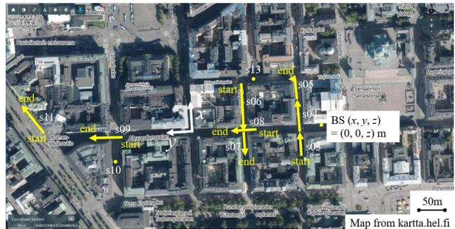
Fig. 3. Dynamic MIMO channel sounding at 5.3 GHz in a downtown Helsinki. A location of the BS along with MS routes s03–s11 are overlaid.
