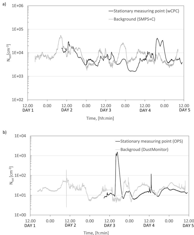
**Figure 2.** Nanoparticle (a) and fine particle (b) concentrations in WP2 measured from the AM room (black line) and from the background (gray line). Water-based condensation particle counter N-WCPC3788 measures particles in the size range from 2.5 nm to 3  $\mu\text{m}$ . Scanning Mobility Particle Sizer SMPS+C measures particles from 5.5 to 350 nm. Optical particle counters OPS3330 measures particles from 300 nm to 10  $\mu\text{m}$  and DustMonitor 1.109 from 265 nm to 31  $\mu\text{m}$ .
