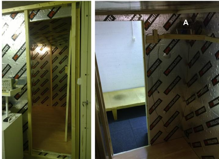
**Fig. 2.** Radio-frequency shielded test room. The entrance to the test room (left), and an internal view of it (right). The radar sensor (A) is placed in the test-room corner in a pointing downwards position.
