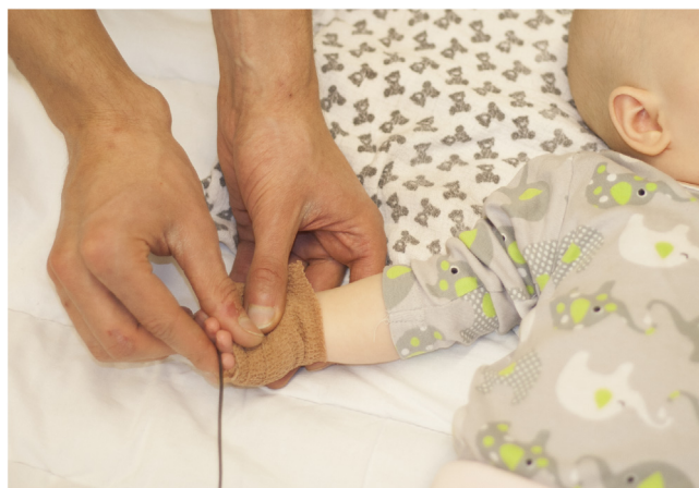
Fig. 1. Stimulation setup. The experimenter is moving the right-hand fingers of the infant. The accelerometer is attached to the fingers with bandage, and its black cable is visible. The situation was set up for illustrative purposes only, and the infant in the picture did not participate in the study.
