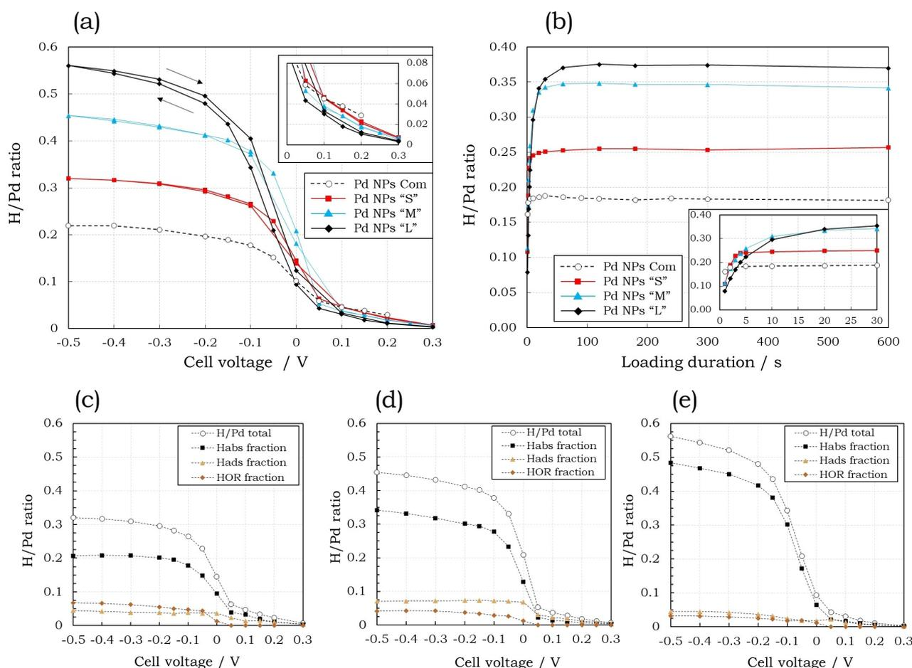
**Figure 3.** Cell voltage dependency (a) and loading duration dependency (b) on the H/Pd ratio measured from the electrochemical desorption curves. Separation of the different H fractions participating to the H/Pd ratio according to [23], Pd NPs "S" (c), Pd NPs "M" (d) and Pd NPs "L" (e). H<sub>2</sub> and N<sub>2</sub> flowrates 50 mL·min<sup>-1</sup>, 30 °C, 120 s loading duration (a, c, d, e), -0.1 V loading voltage (b), desorption at +0.4 V for 120 s.
