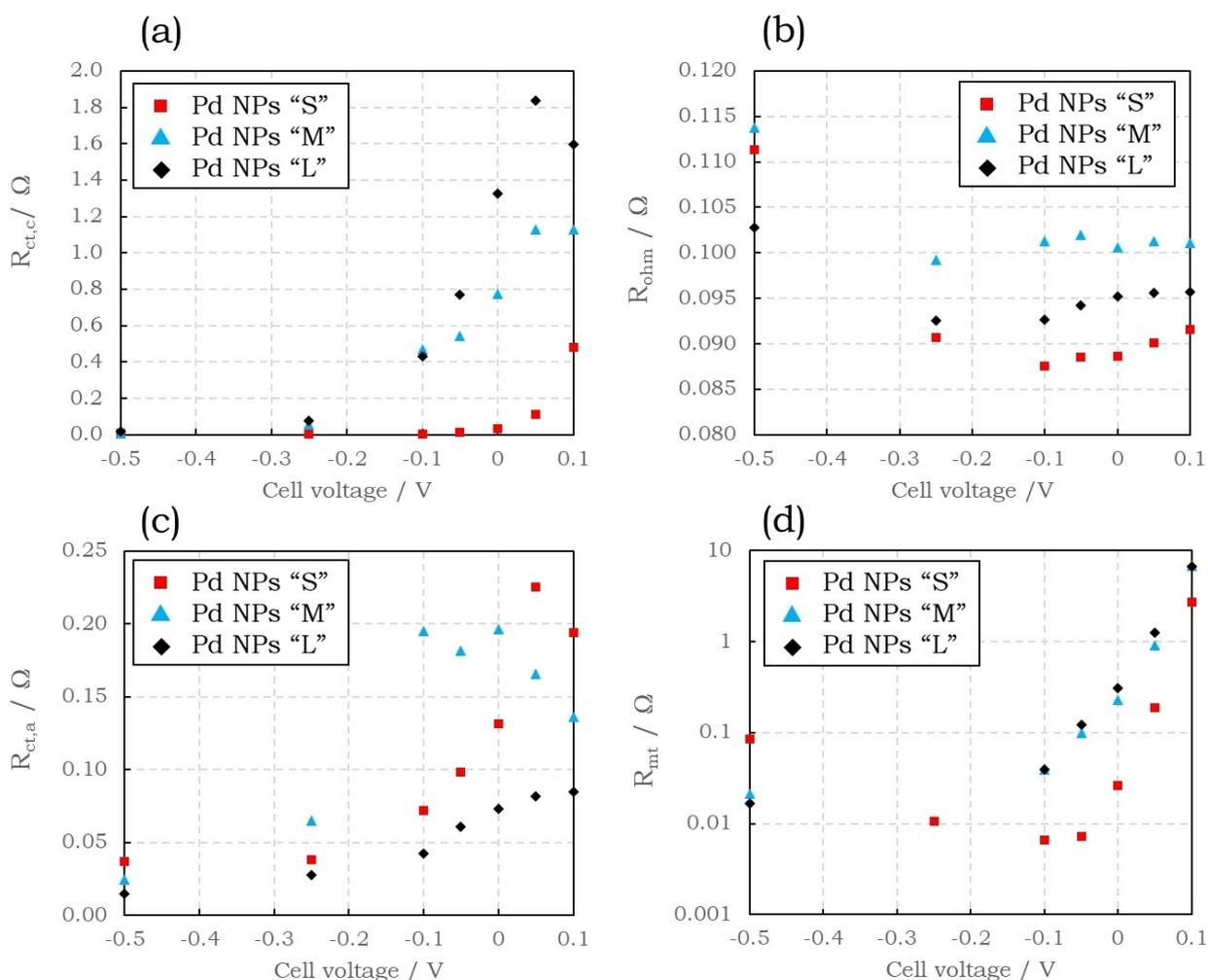
**Figure 6.** Voltage dependency of the cathodic charge transfer resistance (a), ohmic resistance (b), anodic charge transfer resistance (c), and mass transfer resistance (d) extracted from the modelling of the EIS data.  $H_2$  and  $N_2$  flowrates  $50 \text{ mL min}^{-1}$ ,  $30^\circ\text{C}$ , 20 min of stabilization at set potential, 20 mV fluctuations.
