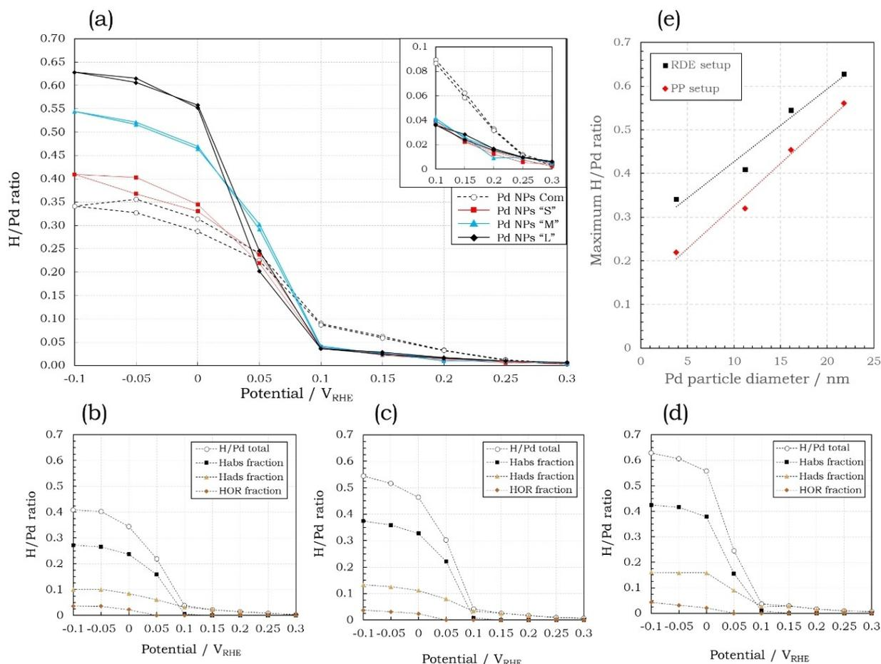
**Figure 4.** Potential dependency of the H/Pd ratio measured from the electrochemical desorption curves in the RDE setup (a). Separation of the different H fractions participating to the H/Pd ratio according to [23], Pd NPs "S" (b), Pd NPs "M" (c) and Pd NPs "L" (d).  $H_2SO_4$  0.5 M, 25 °C,  $N_2$  bubbling, 120 s loading duration, desorption at +0.4 V for 120 s. Particle diameter dependency of the H/Pd ratios measured at  $-0.1 V_{RHE}$  (RDE setup) and at  $-0.5 V$  (PP setup) (e).
