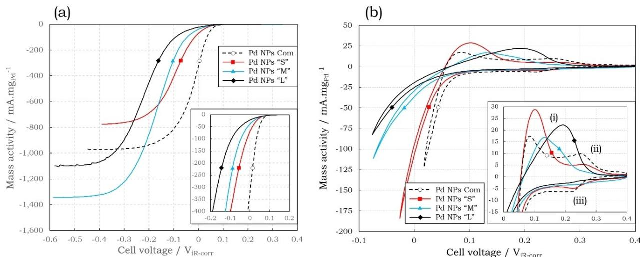
**Figure 5.** Linear sweep voltammograms recorded at 30 °C, with an  $H_2$  and  $N_2$  flowrates of  $50 mL \cdot min^{-1}$ , at a scan rate of  $2 mV \cdot s^{-1}$  (a); cyclic voltammograms recorded at 30 °C, with an  $H_2$  and  $N_2$  flowrates of  $50 mL \cdot min^{-1}$ , at a scan rate of  $25 mV \cdot s^{-1}$  (b). All voltages are  $iR$ -corrected.
