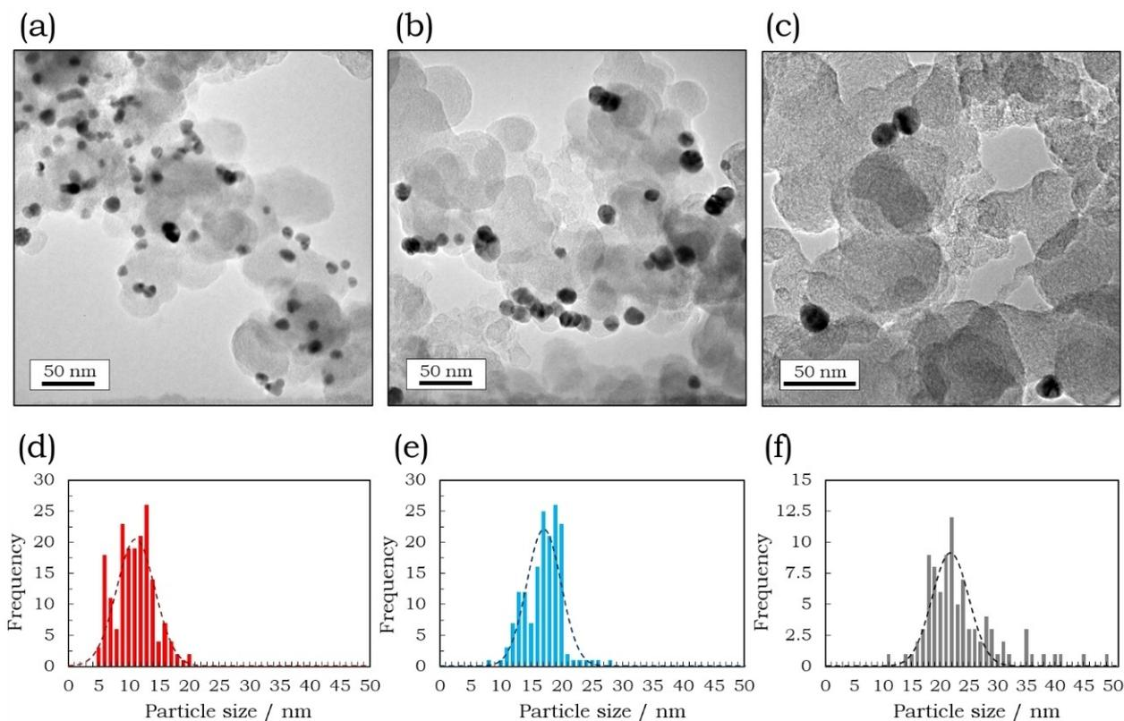
**Figure 1.** Typical micrography of the three prepared samples (a) Pd NPs "S" ( $11.2 \pm 3.2$  nm), (b) Pd NPs "M" ( $17.1 \pm 2.8$  nm) and (c) Pd NPs "L" ( $21.5 \pm 3.2$  nm). Particle size distributions of (d) Pd NPs "S" (180 particles), (e) Pd NPs "M" (165 particles) and (f) Pd NPs "L" (92 particles). The dotted lines correspond to the normal distribution fittings.
