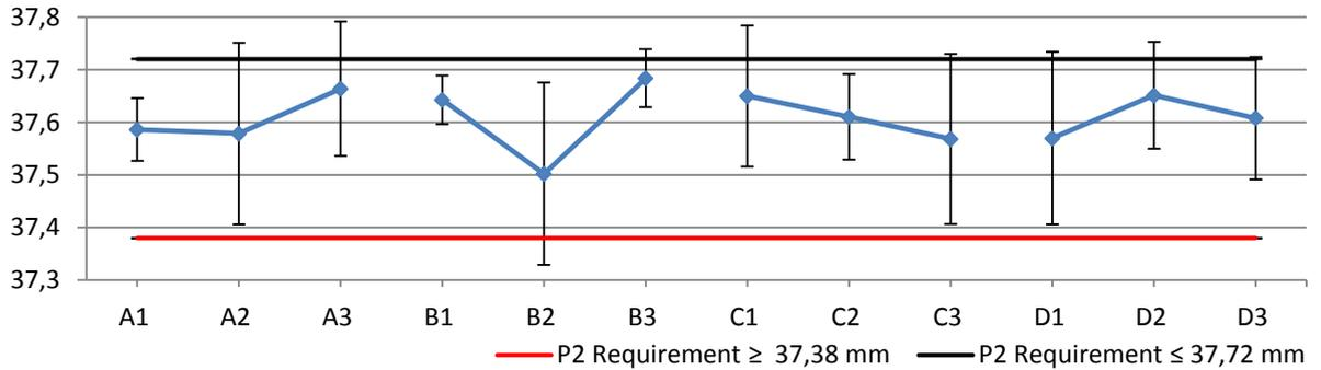
Fig. 6. Response graphic of the performance variable P2 (Hole to hole distance)
