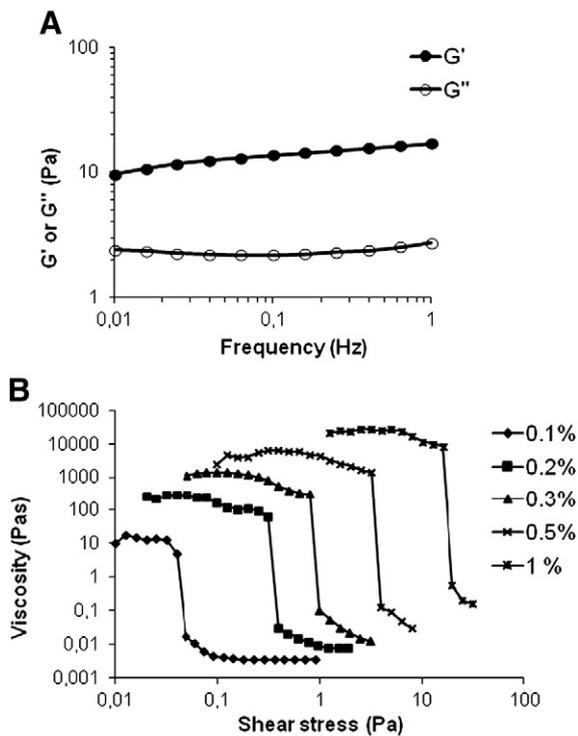
Fig. 2. Rheological properties of nanofibrillar cellulose hydrogel. (A) Frequency dependence of storage ( $G'$ ) and loss modulus ( $G''$ ) of a 0.5 wt.% hydrogel. (B) Flow curves of 0.1–1 wt.% hydrogel as function of shear stress.
