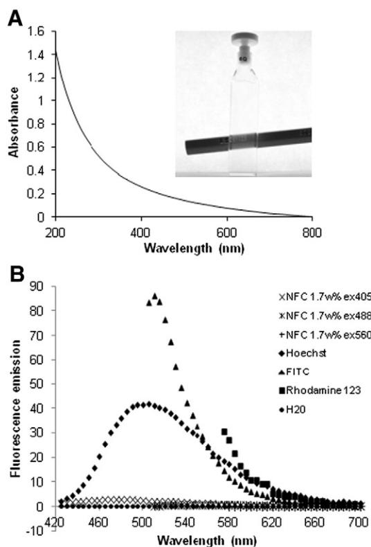
**Fig. 5.** (A) Absorbance spectrum of 0.5 wt.% NFC hydrogel at the UV–visible wavelengths. The inset image visualizes the transparency of the hydrogel in the measurement cuvette. (B) Fluorescence spectra of hydrogels compared to purified water at excitation wavelengths of commonly used molecular probes (405, 488 and 560 nm).
