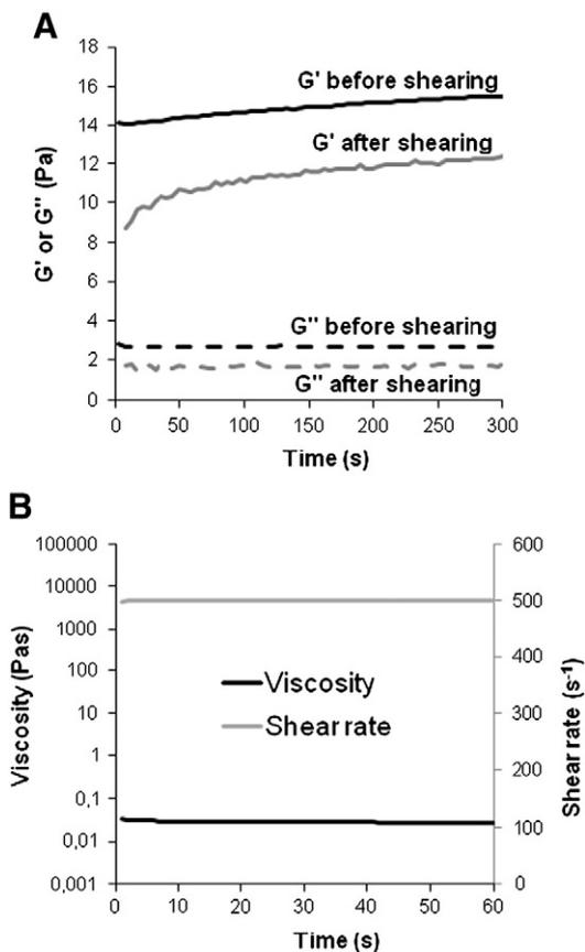
Fig. 3. (A) Structure of 0.5 wt.% nanofibrillar cellulose hydrogel recovers after high-speed ( $500 \text{ s}^{-1}$ ) shearing. (B) Evolution of viscosity when a 0.5 wt.% NFC gel was sheared at a constant shear rate of  $500 \text{ s}^{-1}$ .
