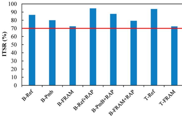
Figure 7. ITSR results on the different mixtures.
