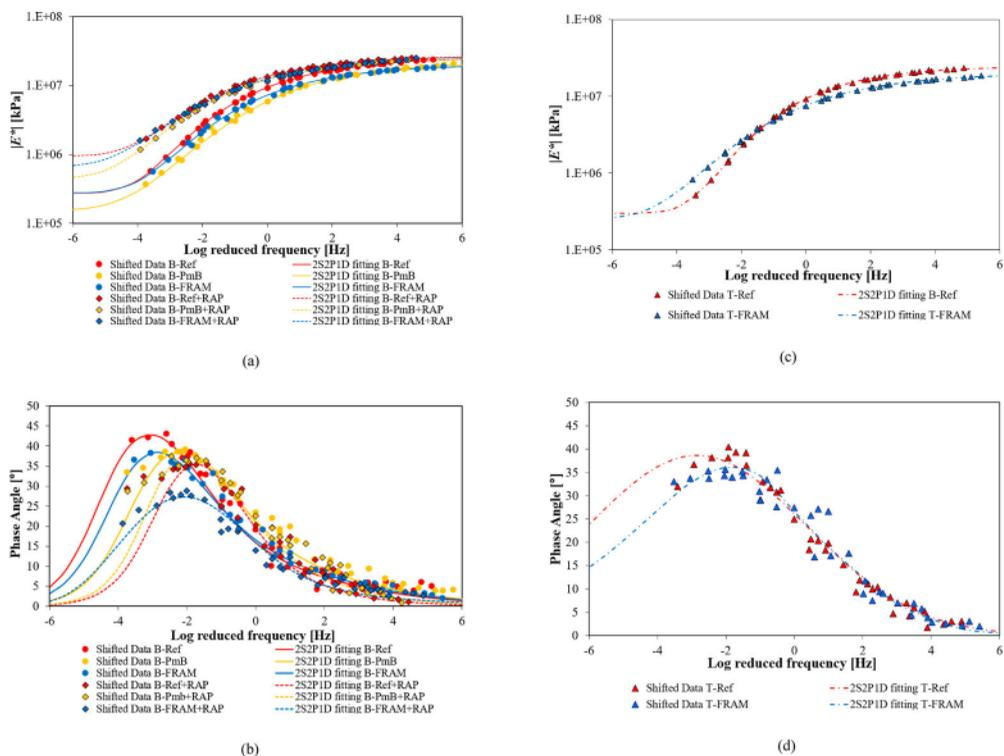
**Figure 8.** Master curves of the mixtures at a reference temperature of 10°C: (a) binder layer complex modulus  $|E^*|$ ; (b) binder layer phase angle  $\delta$ ; (c) base layer complex modulus  $|E^*|$ ; (d) base layer phase angle  $\delta$ .
