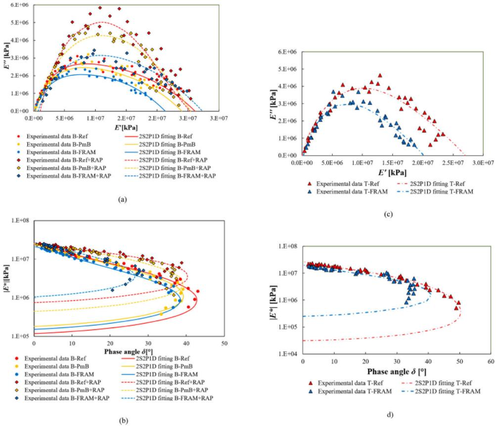
**Figure 9.** Experimental data and 2S2P1D fitting displayed in (a) binder layer Cole-Cole plot; (b) binder layer black-diagram; (c) base layer Cole-Cole plot; (d) base layer black-diagram.
