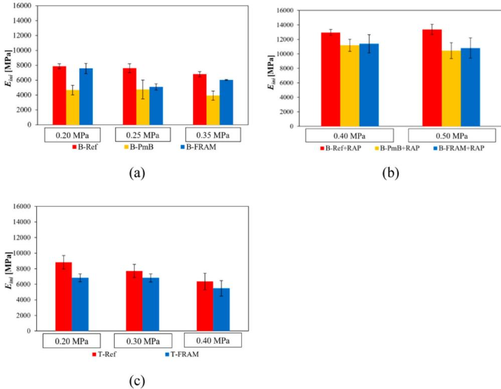
**Figure 11.** Initial stiffness at the same stress levels: (a) binder layers’ mixtures without RAP; (b) binder layers’ mixtures containing RAP; (c) base layers’ mixtures.
