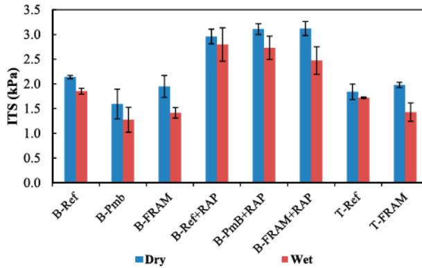
**Figure 6.** Indirect Tensile Strength results.
