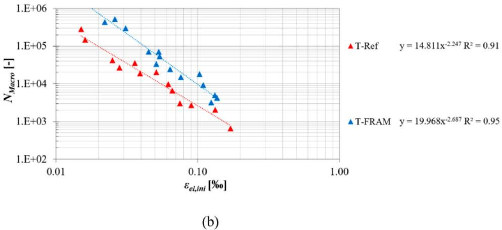
**Figure 10.** Fatigue results at 20°C: (a) binder layers mixtures with and without RAP; (b) base layers mixtures.
