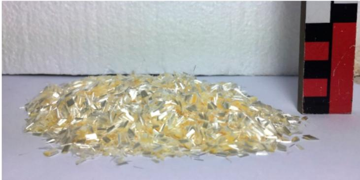
Figure 3. Illustration of PAN fibres.
