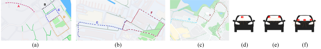
Fig. 5. Data collection trajectories and camera placements. Fig. 5 (a) illustrates the trajectories A, B, C, and D in a residential area. Fig. 5 (b) and (c) depict trajectories E, F, and G on a university campus. Fig. 5 (d)–(f): the different configurations of camera placements: single view versus double view versus triple view.
