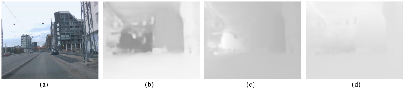
Fig. 4. Illustrative examples of the output of the BTS network. (a) RGB image. (b) Depth prediction. (c) Lateral prediction. (d) Height prediction.
