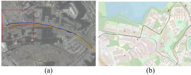
Fig. 7. (a) Estimated by SfM camera positions of each image in data set III (camera 1 in blue and camera 2 in yellow) versus the ground truth obtained with RTK technology (in red). (b) Camera poses of data set VI estimated by SfM (green) versus the path extracted from Google Maps for comparison (red solid line), the red numbers specify the locations of example images in Fig. 8.
