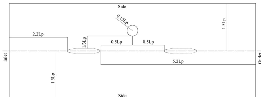
**Figure 2.** Top view of the Numerical Wave Tank and positions of the ship and ice floe.
