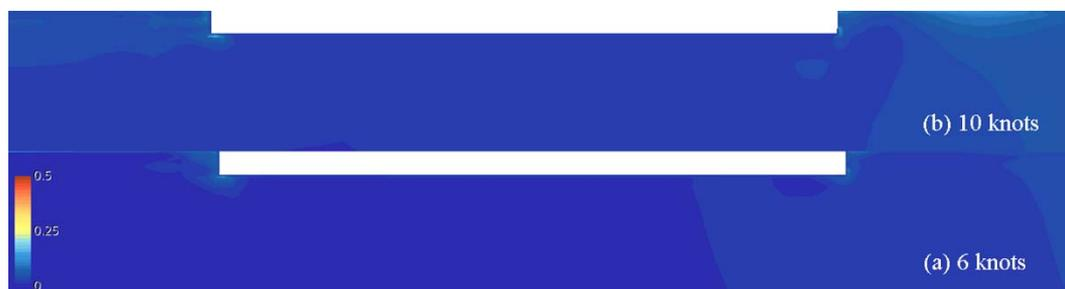
**Figure 6.** Fluid velocity field at the transverse section crossing the center of ice floe.
