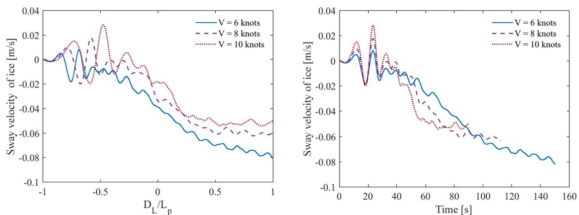
**Figure 5.** Sway velocity of the ice floe under the waves generated by the passing ship.
