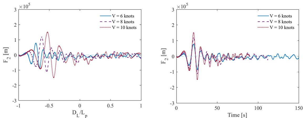
**Figure 7.** Transient fluid force in sway on the ice floe.
