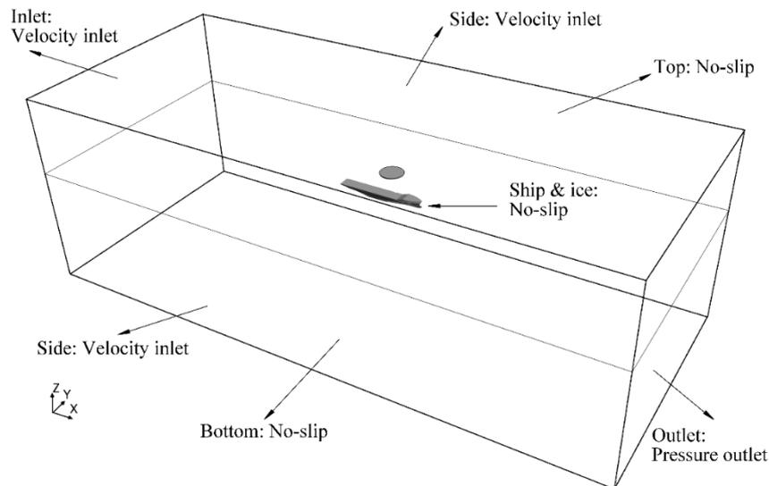
**Figure 1.** 3D view of Numerical Wave Tank and its boundary conditions.
