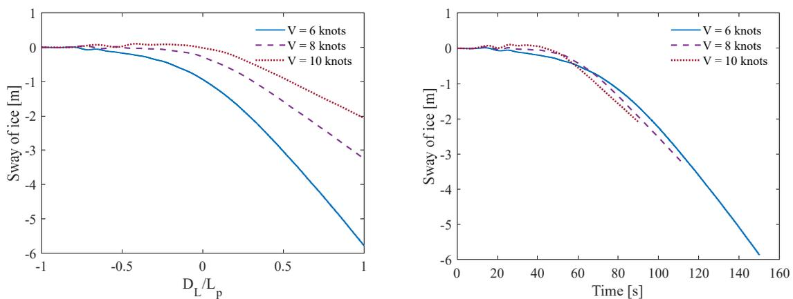
**Figure 4.** Sway of the ice floe under the waves generated by the passing ship.
