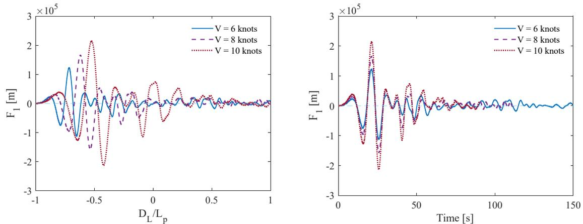
**Figure 10.** Transient fluid force in surge on the ice floe.
