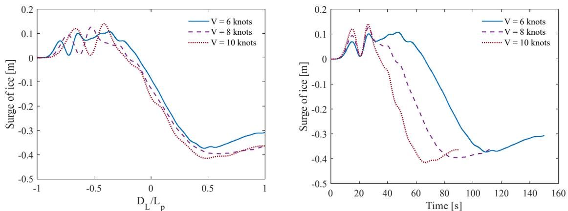
**Figure 8.** Surge of the ice floe under the waves generated by the passing ship.
