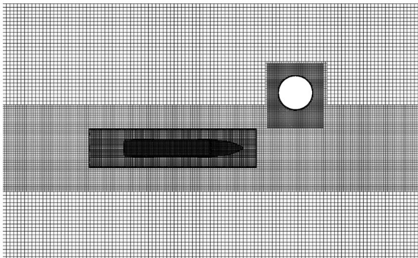
**Figure 3.** Trimmed mesh in the fluid domain.
