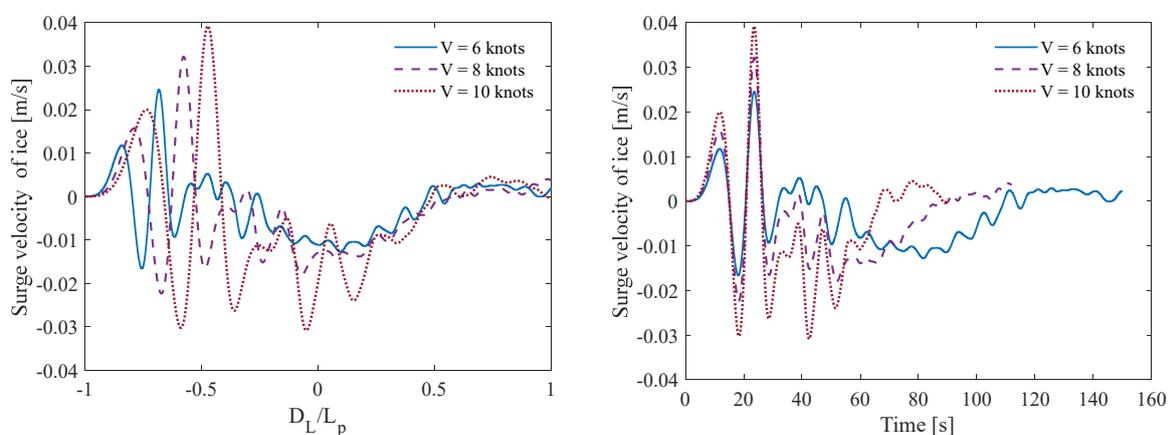
**Figure 9.** Surge velocity of the ice floe under the waves generated by the passing ship.
