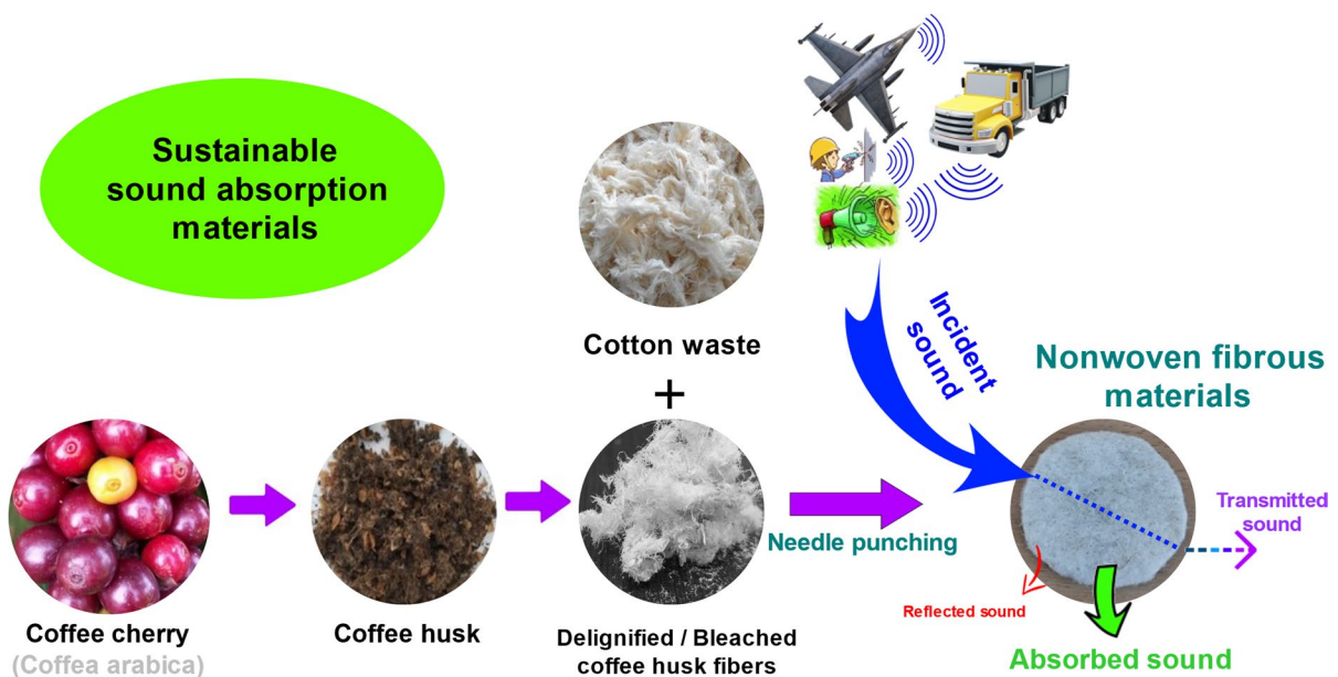
Fig. 1 Various stages to prepare sustainable sound absorption nonwoven materials
