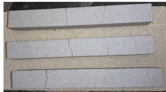
**Figure 12. Cracks developed in test bars when Sil-E test bars were heated to 900 °C.**
