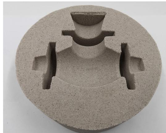
**Figure 3. One mold prepared using silica and Binder C (Sil-C mold).**
