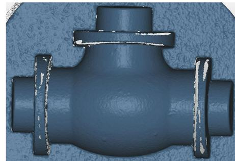
**Figure 25.** 3D scan of Sil-E mold made with 3D-printed thermal-resistant plastic pattern.
