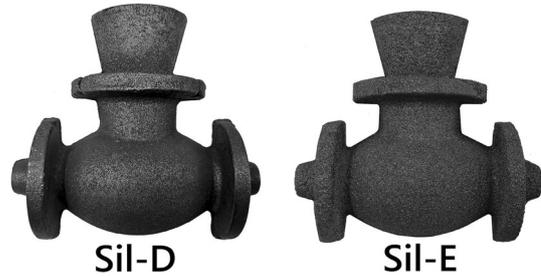
**Figure 16.** On the left Sil-D casting and on the right Sil-E casting.
