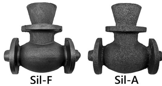
**Figure 15.** On the left Sil-F casting and on the right Sil-A casting.
