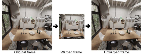
Figure 1: Example of a rendered frame (left) warped with a foveated radial warp (FRW) function (center) and inversely warped back to original shape (right). The gaze fixation point is at the center of the frame.
