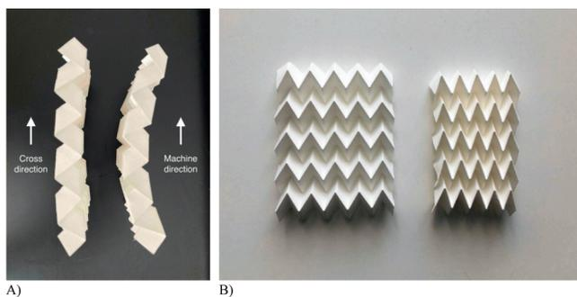
**Fig. 3.** A) Miura-ori folded perpendicular (CD) vs. parallel to machine direction (MD), B) Miura-ori in two different 200 g/m<sup>2</sup> materials (photos by Miia Palmu).
