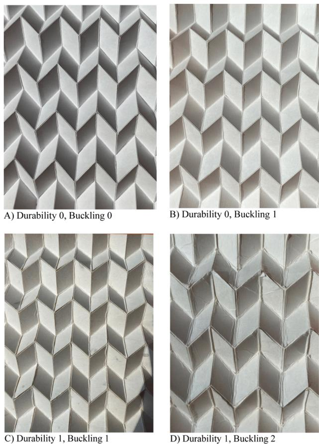
Fig. 9. Reference pictures for Durability (0/1) and Buckling (0/1/2).
