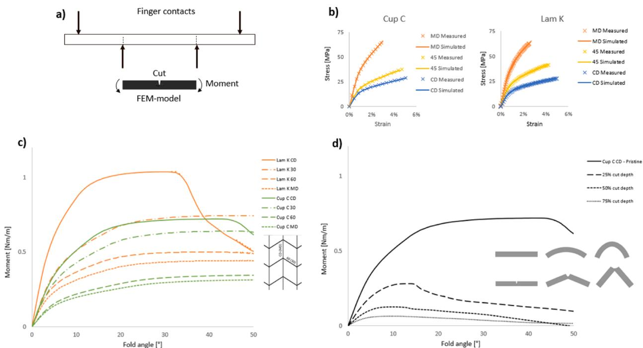
Fig. 5. A) Simulation setup; B) Material model calibration; C) Simulated response (moment versus fold angle) for fold lines with different material orientations; D) Effect of pre-cut depth.
