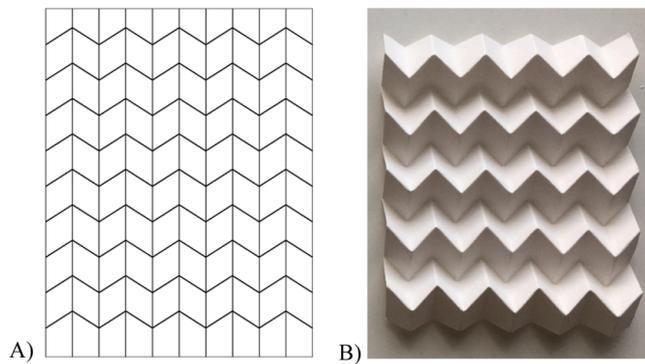
Fig. 1. A) a 2D Miura-ori tessellation pattern applied to the samples, B) a folded board sample with the Miura-ori tessellation (figures by Miia Palmu).
