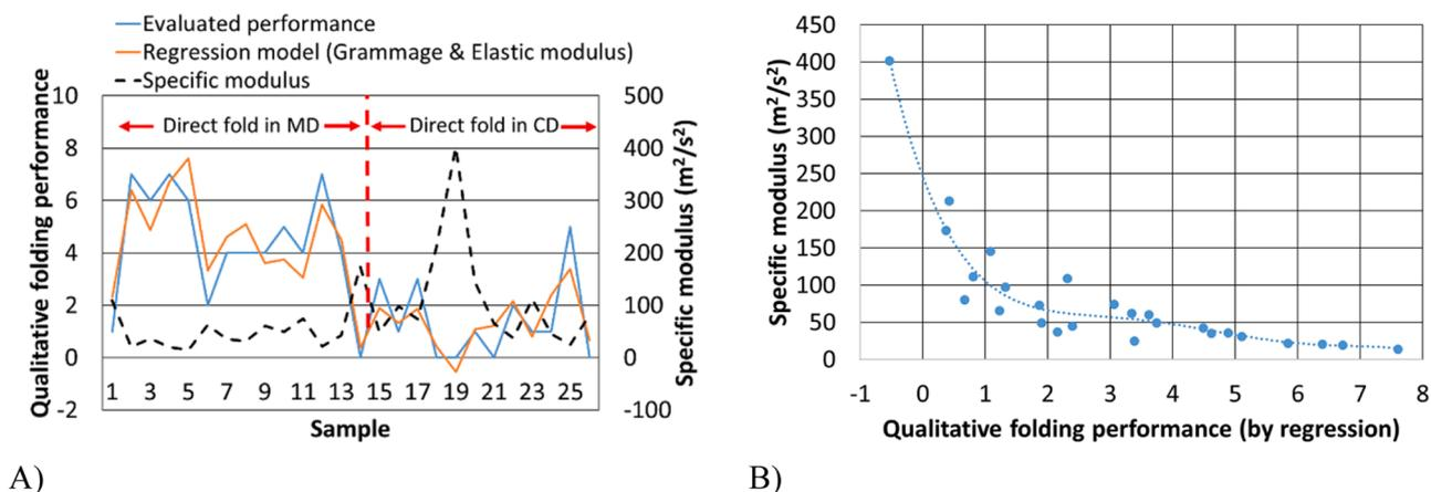
Fig. 4. A) Qualitative folding performance of the studied samples. Evaluated performance and linear regression for performance (applying direction of straight folding, grammage and elastic modulus in the direction of straight folding of the samples). B) Specific modulus as a function of qualitative folding performance given by the linear regression model.
