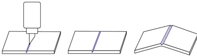
**Fig. 2.** Schematic presentation of kiss-cutting the Miura-ori tessellation pattern and folding of the samples.
