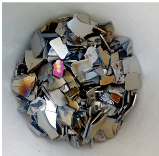
Figure 2. Broken magnets after demagnetization used as a feed in the leaching process.
