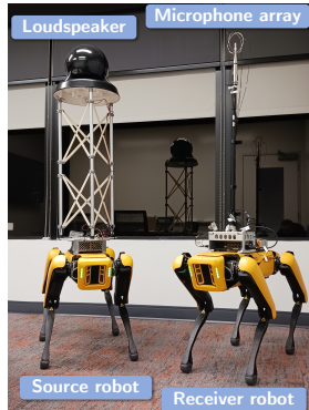
Figure 1: Robot system used in the evaluation. It contains two Boston Dynamic Spot robots, equipped with a loudspeaker and a microphone array, respectively.
