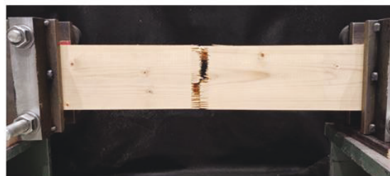
Figure 2: FJ after failure in a tensile test
