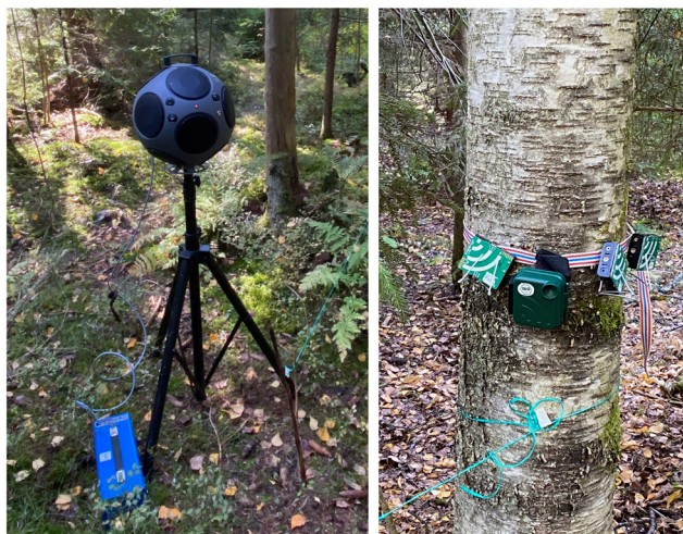
FIG. 2. (Color online) The applied battery driven omnidirectional sound source and AudioMoth microphones with and without the case.
