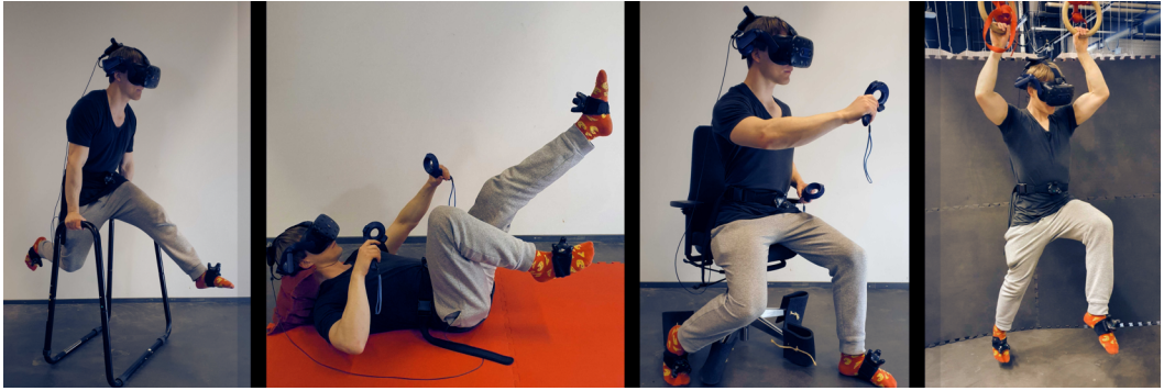
Fig. 3. All the four non-standing locomotion approaches we explored. All these share the design principle that one’s weight is not supported by the legs. Thus, one can perform walking, running, strafing, and jumping movements in the air or only slightly touching the ground with their feet, without being limited by a small physical space.
