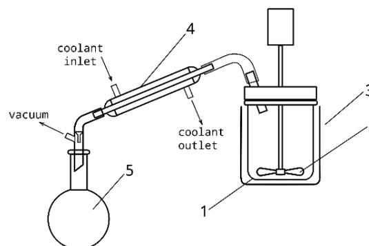
**Figure 2.** Experimental setup used for CC and EC studies. (1) Reactor, (2) stirrer, (3) jacket, (4) cooling system, (5) water collector.
