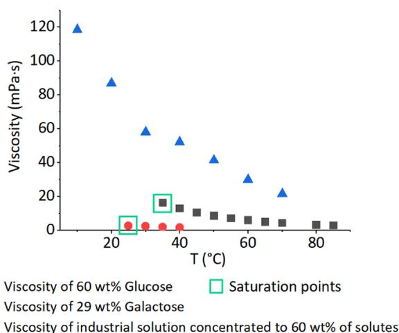
**Figure 5.** Measured viscosities of the pure glucose and galactose solution and the concentrated industrial side stream.
