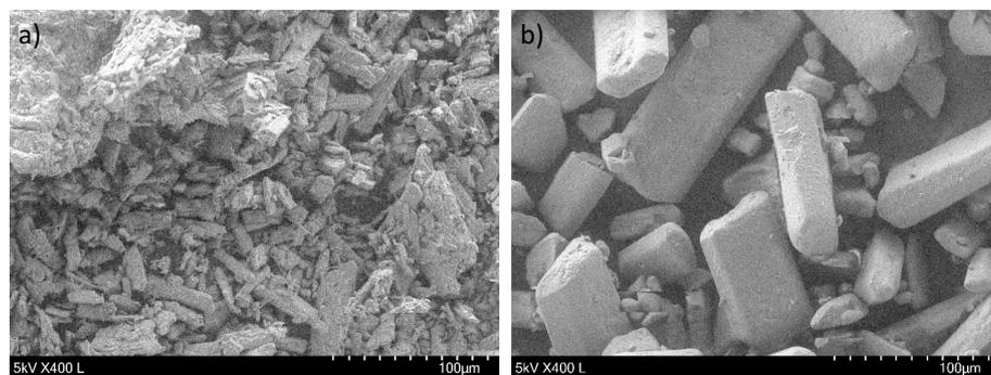
**Figure 7.** Typical SEM micrographs of (a) D-galactose crystallized from the industrial side stream using fast cooling from 50 to 15 °C and from 15 to 5 °C with a cooling rate of 2 K h<sup>-1</sup>, and a total batch time of 5.3 h (experiment no. 10) (400-fold magnification, scale bar 100 μm), and (b) pure water (400-fold magnification, scale bar 100 μm).
