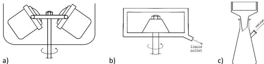
Figure 3. Separation systems: (a) benchtop centrifuge, (b) basket centrifuge, (c) Büchner funnel.
