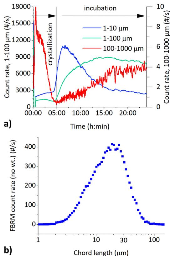
**Figure 8.** FBRM result of CCSTD with a two-stage cooling program and 20 h of incubation. (a) FBRM graph and (b) final unweighted chord length distribution.
