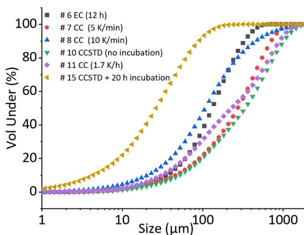
**Figure 6.** Cumulative particle size distribution curves obtained by laser diffraction analysis.
