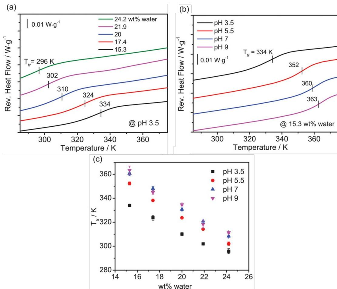
**Figure 6.** Reversing heat flow curves of (a) (PAH/PAA)<sub>3.5</sub> complexes of varying water content and of (b) varying complexation pH values and constant water content (15.3 wt. % water). For (a) and (b), second heating scans are shown, and curves have been shifted along the y-axis for clarity. (c)  $T_{tr}$  for PAH/PAA complexes for varying complexation pH values and water content. Reprinted (adapted) with permission from ref. <sup>67</sup> Copyright 2016 American Chemical Society.
