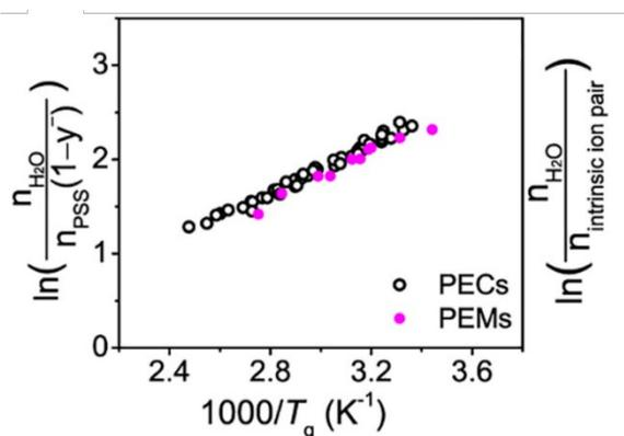
**Figure 4.** A plot of  $\ln(n_{H_2O} / n_{\text{intrinsic ion pair}})$  vs  $1000/T_g$  for PDADMA/PSS polyelectrolyte complexes (PECs, black circles) and polyelectrolyte multilayers (PEMs, pink circles). Reprinted (adapted) with permission from ref. <sup>66</sup> Copyright 2018 American Chemical Society.
