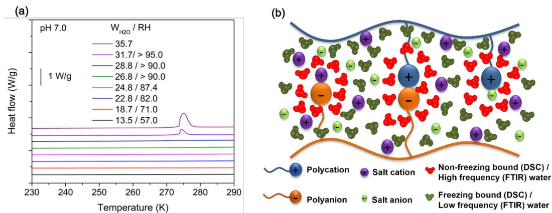
**Figure 10.** (a) DSC heat flow curves for PAH/PAA PECs at pH 7.0 with varying water content. Adapted with permission from ref. <sup>88</sup> Copyright 2021 American Chemical Society. (b) Water microenvironments in polyelectrolyte complexes and multilayers as identified by DSC and ATR-FTIR spectroscopy. Reproduced from ref.<sup>56</sup> with permission from the Royal Society of Chemistry.
