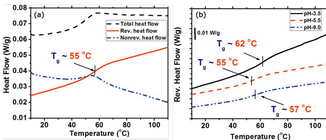
**Figure 5.** (a) MDSC thermograms of hydrated PAH/PAA LbL films assembled from pH 5.5 solution. (b) Reversing heat flow curves for hydrated PAH/PAA LbL films assembled from pH 3.5, 5.5, and 9.0 solutions. Curves in (b) have been shifted along the  $y$ -axis for clarity. Heating rate at 2 °C min<sup>-1</sup>, amplitude of 1.272 °C, and period of 60 s (second heating cycle shown). Reprinted (adapted) with permission from ref. <sup>58</sup> Copyright 2012 American Chemical Society.
