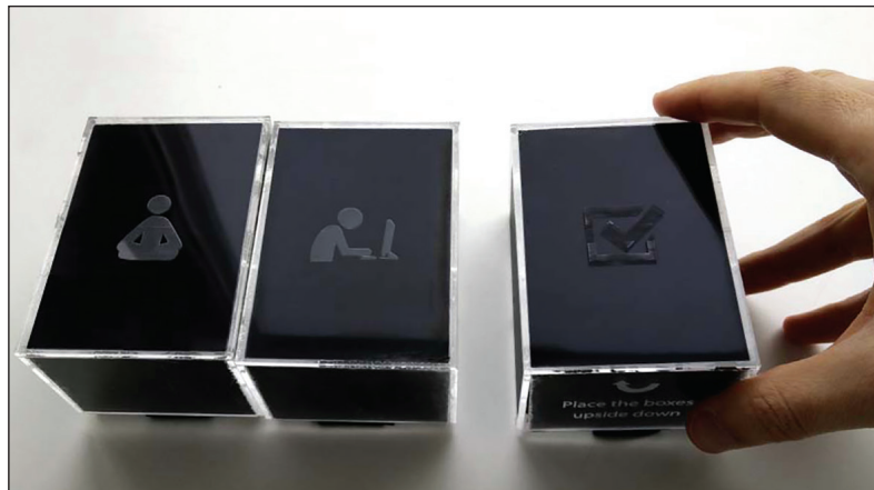
Figure 2: To connect the Feeler smart objects, the user needs to place them next to each other.
