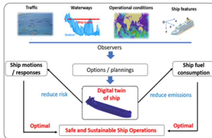
Figure 6: The iterations of digital twins for safe and sustainable ship operations.
