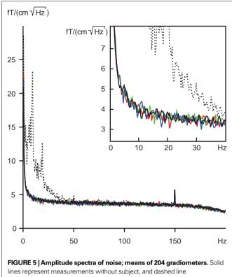
measurement with subject. Black, no eye tracker; blue, green and red lines, eye tracker at 100, 117 and 140 cm distance from the measurement helmet. Insert focuses on the frequency range of 0–40 Hz.
