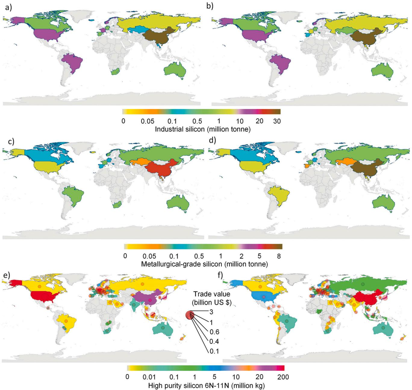
Fig. 2. Global mass flow of silicon (tonne) in 10-year intervals (between 2010 and 2030) and trade of high-purity silicon (6N–11N) (kilogram) in 2021. a, Cumulative industrial silicon in the period 2010–2020. b, Cumulative industrial silicon in the period 2020–2030. c, Cumulative metallurgical grade silicon in the period 2010–2020. d, Cumulative metallurgical grade silicon in the period 2020–2030. e, Export of high-purity silicon in 2021. f, Import of high-purity silicon in 2021.
