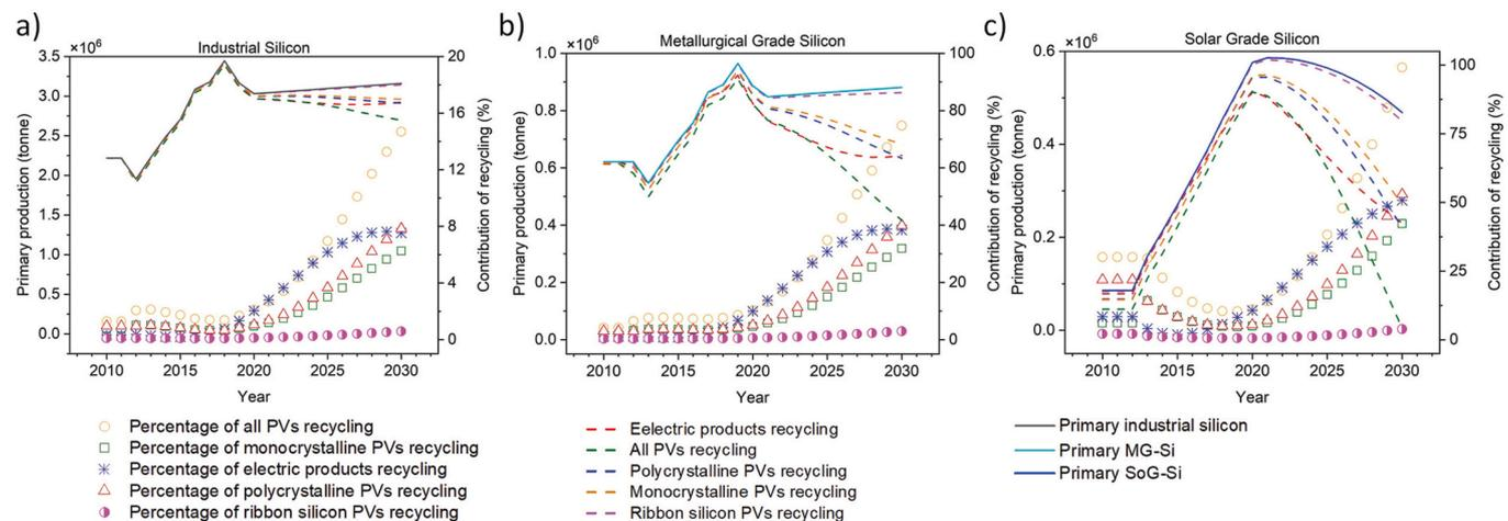
**Fig. 6.** The impact of circularity of silicon on its primary production between 2010 and 2030. **a**, Annual global industrial silicon production. **b**, Annual global metallurgical grade silicon production. **c**, Annual global solar grade silicon production.
