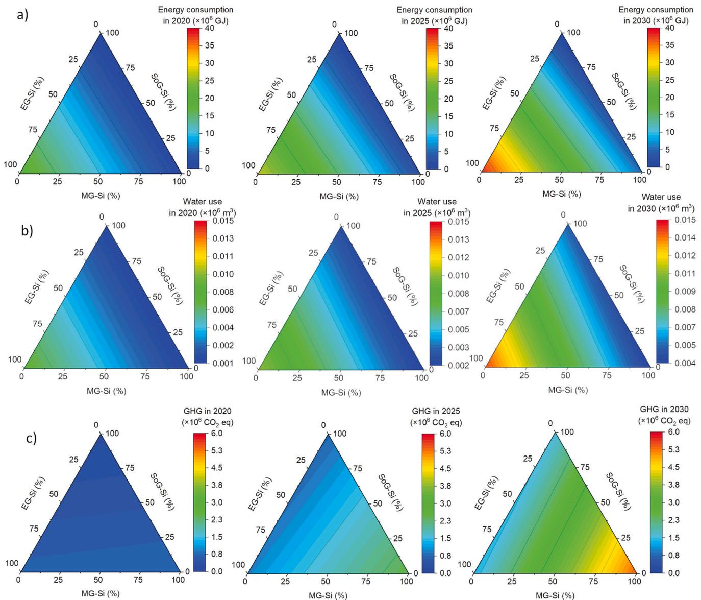
**Fig. 12.** Environmental impact of silicon recovery by integrating its circularity flows between 2020 and 2030 (Scenarios: 0–100%). a, Energy consumption, in gigajoules (GJ). b, Water use, in cubic meters. c, GHG emissions, in tonnes CO<sub>2</sub> eq.
