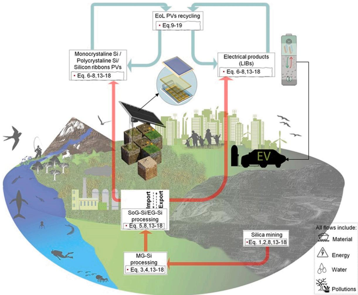
Fig. 1. Conceptual model of silicon flows in green energy technologies.
