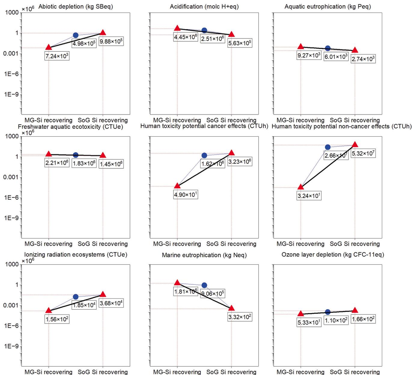
Fig. 11. Environmental effects of the recovering metallurgical and solar grades of silicon by 2030. The blue circle represents the centroid point.
