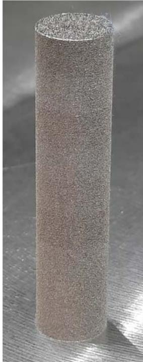
**Figure 2.** Additively manufactured test specimen (316L) with segmented exposure strategies.
