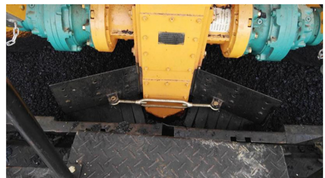
Fig. 72. Installation of rubber baffle in screw gearbox.
