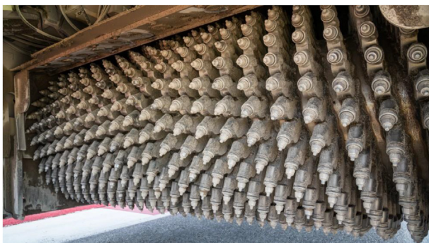
Fig. 75. Fine milling rotor with 672 cutters.
