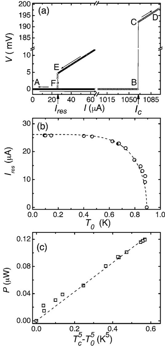
FIG. 2. Electron-phonon coupling experiment (see details in the text). (a) Transition of a Mo resistor from superconducting to normal state ( $A \rightarrow B \rightarrow C \rightarrow D$ ) and from normal to superconducting state ( $D \rightarrow E \rightarrow F \rightarrow A$ ) at  $T_0 = 380$  mK. (b) Dependence of  $I_{\text{res}}$  on bath temperature  $T_0$ . (c) Dependence of heating power on  $T_c^5 - T_0^5$ .
