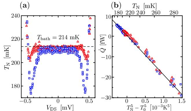
FIG. 3 (color online). (a) Electron temperatures extracted from the data acquired at bath temperature 214 mK with the gate open ( $n_g = 1/2$ , blue squares) and closed ( $n_g = 0$ , red triangles). (b) The theoretical cooling power versus  $T_N^5 - T_0^5$  for each data point of the left panel, and a linear fit to it. According to Eq. (4), the slope is given by  $-\Sigma \mathcal{V}$ .
